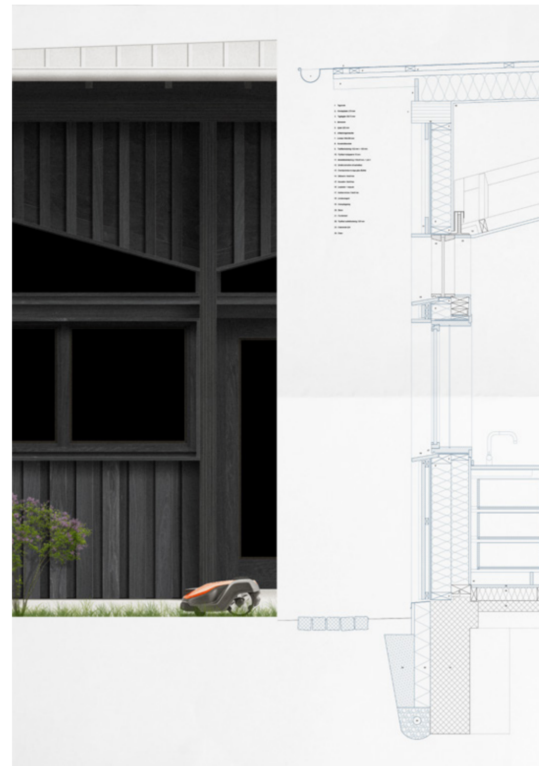
1:15 Section of the new cladding
