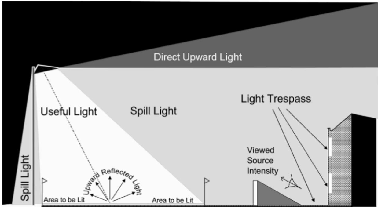
Figure 3: Illustrating lighting efficiency (Guidance Notes for the Reduction of Obtrusive Light 1)
