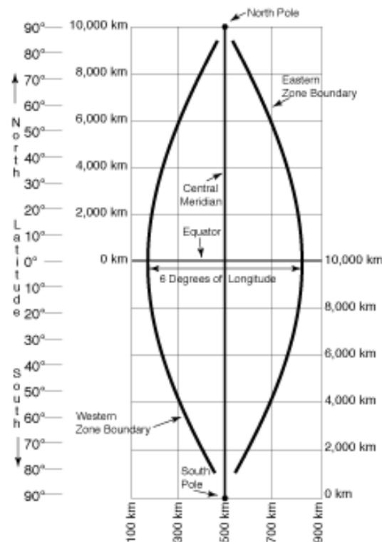
Figure 8: UTM coordinate system diagram (MapTools)
