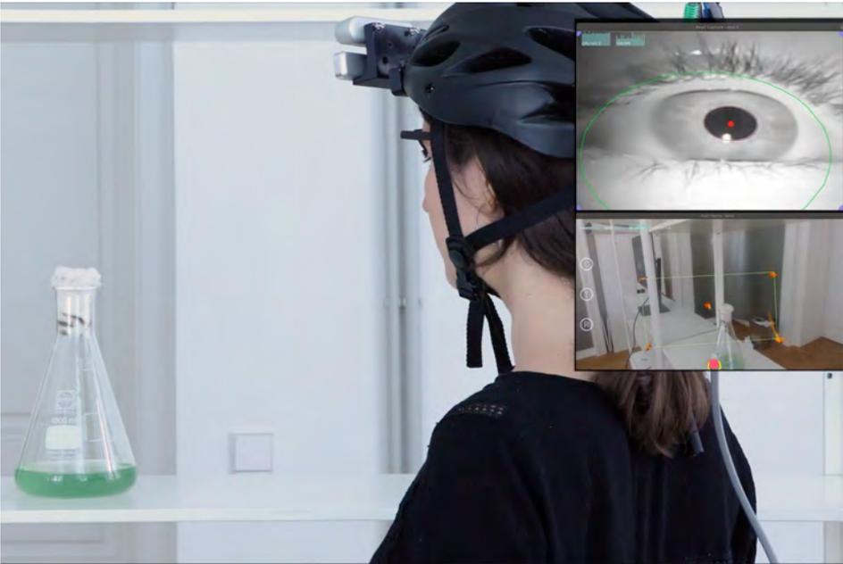
**Figure B.6:** Eye-tracking device (prototype 1) detects the gaze direction and position of the visitor.
