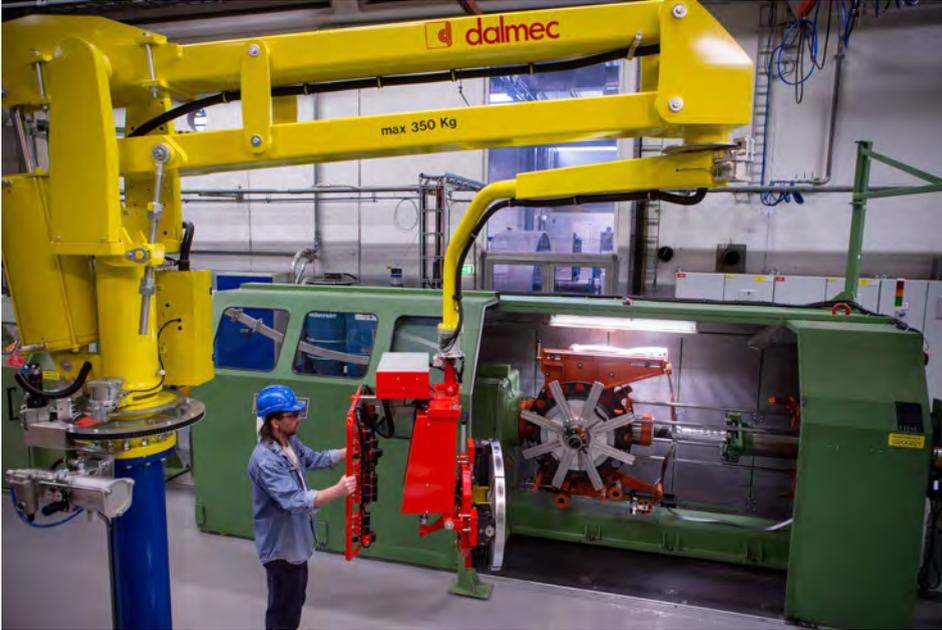
**Figure A.4:** Lift assist device for rolls of metallic banding (photo by Dalmeccan).
