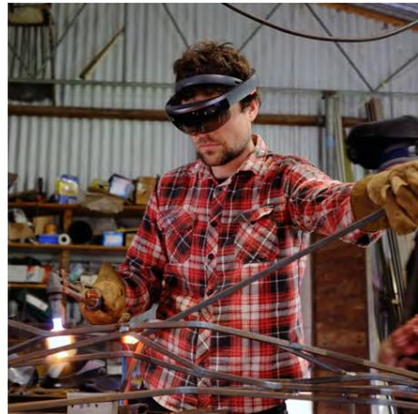
(b) *Fologram* provides AR assistance to instruct craftspeople during fabrication such as welding or bending of steel [67]
