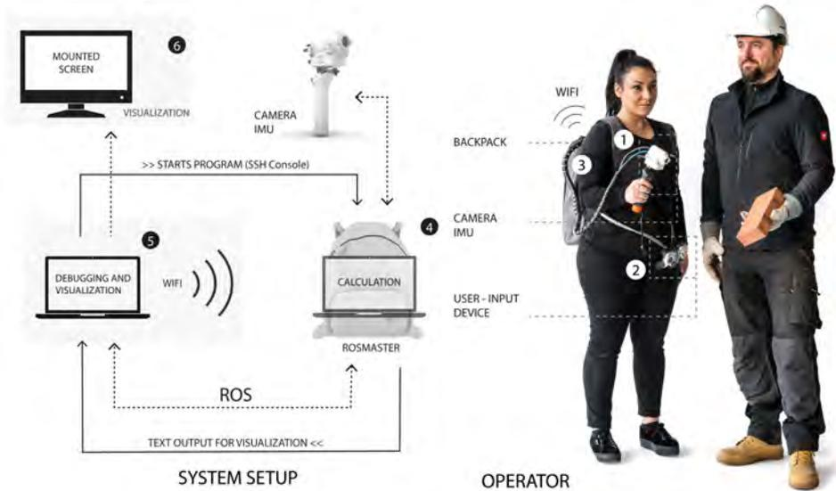
**Figure 3.4:** Custom-built AR setup: operator, bricklayer, handheld camera and IMU (1), portable sensory-input device (2), WIFI connection (3), calculation laptop (4), debugging and visualisation laptop (5), mounted screen (6)
