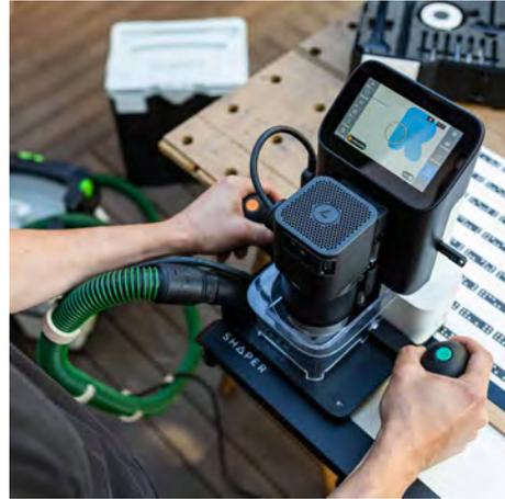
(b) *Shapertool* is a manually controlled CNC router to mill wood precisely and intuitively [66]
