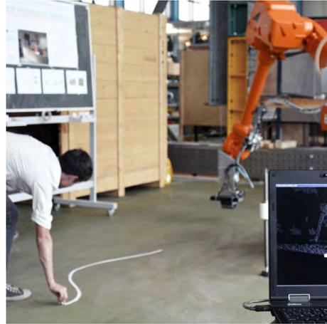
(b) *Endless wall* incorporates spatial input to manipulate the design of a brick wall [82].
