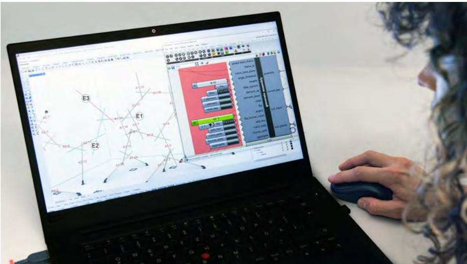
**Figure 3.42:** The user interface of the interactive design model provides input controls for selecting a starting element for a new triplet and defining the triplet's rotation angle via a number slider
