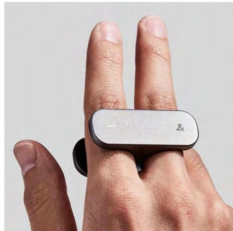
(b) *Litho* is a wearable device that can be clipped between the index and middle finger [194]
