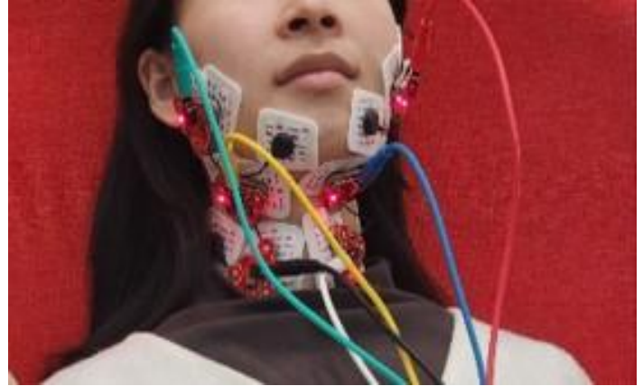
Fig. 4. EMG sensor setup on test subject
