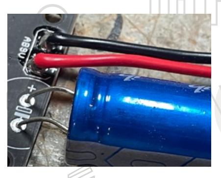
now solder the power wires and the large reserve capacitor, paying close attention to the polarity indicated on the board. 680uf and up will work swell.
