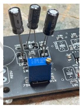
**THEN:** Add the mini trim potentiometer directly below the 10uf caps. This will allow you to bias the power starve waveform toward positive or negative, allowing the board to stay in full powered mode for longer periods of time OR keeping it in starvation for longer. We used these top adjustment mulit-turn potentiometers, but you can use any type that fits (plus some that don't fit by bending legs). You could even wire a full size potentiometer to this spot with wires if you wanted!
