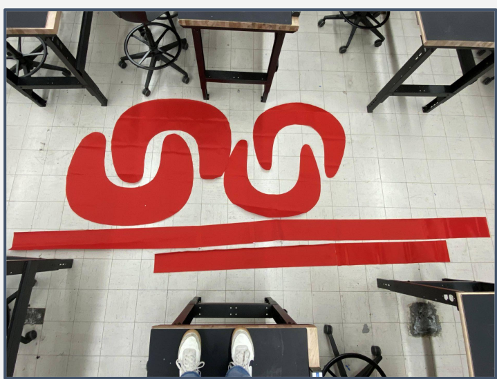
Cut pattern from TPU-coated ripstop
