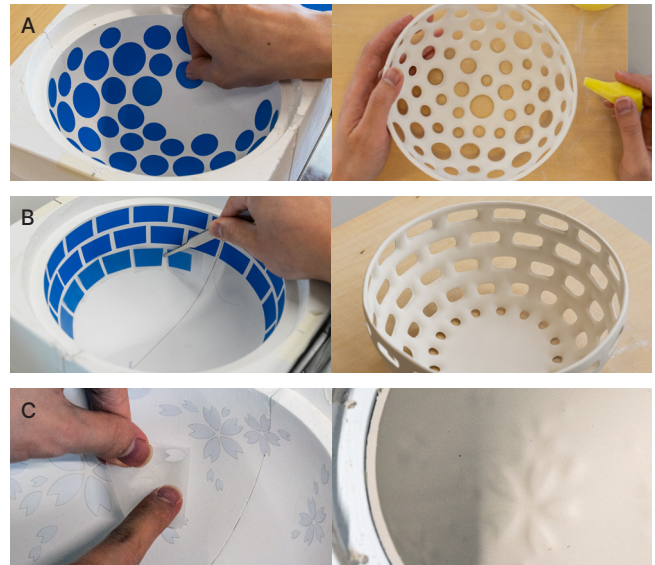
Figure 21: Applying different masks on same bowl mold for different types of holes. A: Varying circles in vinyl. B: Varying rectangles in vinyl. C: Varying sakura petal shapes in paper.
