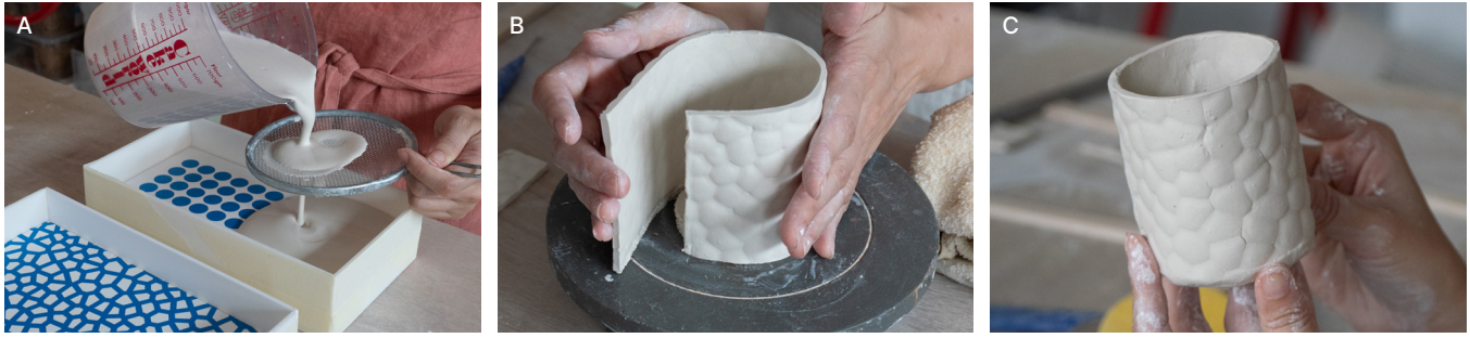
Figure 22: Genevieve making a textured ceramic cup. A: Creating textured ceramic slabs using resist slip-casting. B: Hand-shaping the textured ceramic slab into a cylinder form. C: Finished ceramic cup featuring intricate Voronoi texture.
