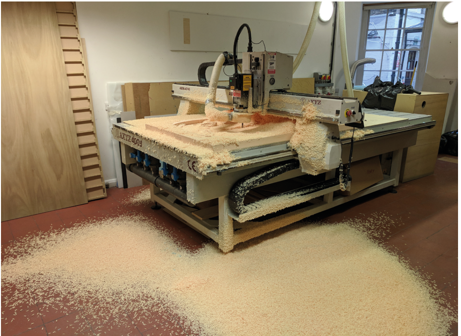
AA Digital Prototyping Lab, Milling Mayhem , CNC milling of a medium-density block.
