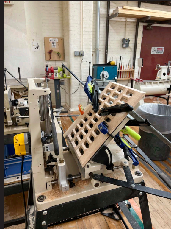
my initial plan to make a hidden spline and ended up forgot to set the depth and cut through the wood...
