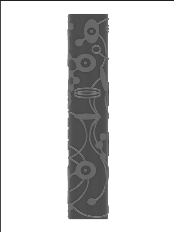
discover .FlowAlongSrf command in Rhino and wrap the map around cylinder
