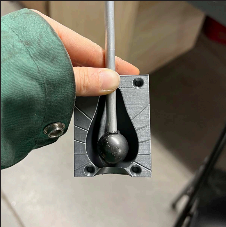
pendulum mold for resin-casting (with the help from Jack!)
