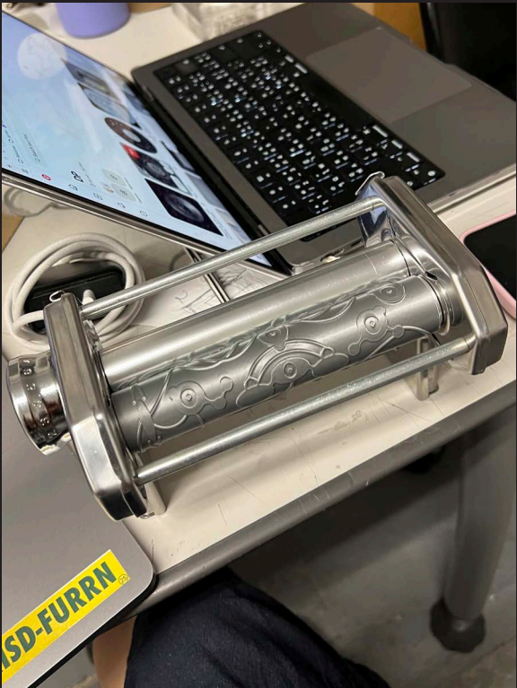
insert the 3D printed embossing tube into the machine
