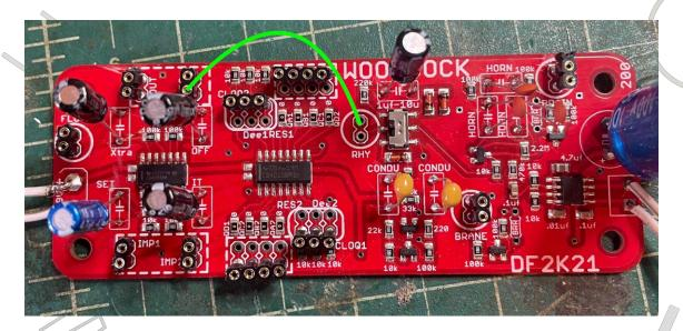
A note on the XTRA oscillator and the FLUT input: XTRA oscillator is a NAND oscillator with FLUT as the inhibitory input. Meaning you can patch an oscillator or other signal into FLUT to get more complex gated rhythms and oscillations. Be careful tho! If nothing is connected to FLUT, XTRA output will behave erratically.
