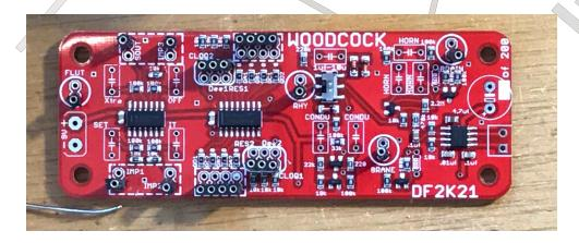
Once you have collected all the requisite parts, start by soldering the pin headers for connections in the various elements of the bird brain.
