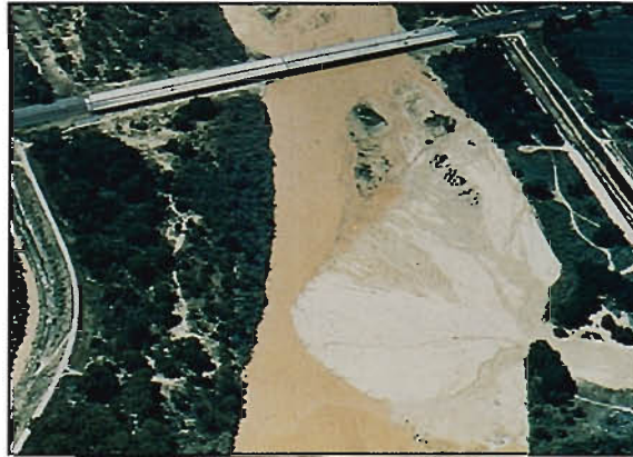
Sediment plug in the Rio Grande carried by rain in the Calabacillas Arroyo, August, 1988
