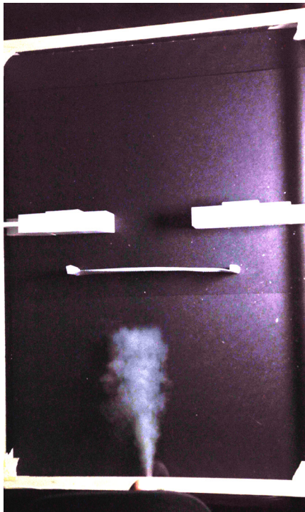
1:20 AIR DUCT TESTS SEQUENCE:1, NET OUTSIDE FACADE 0:06 min.
