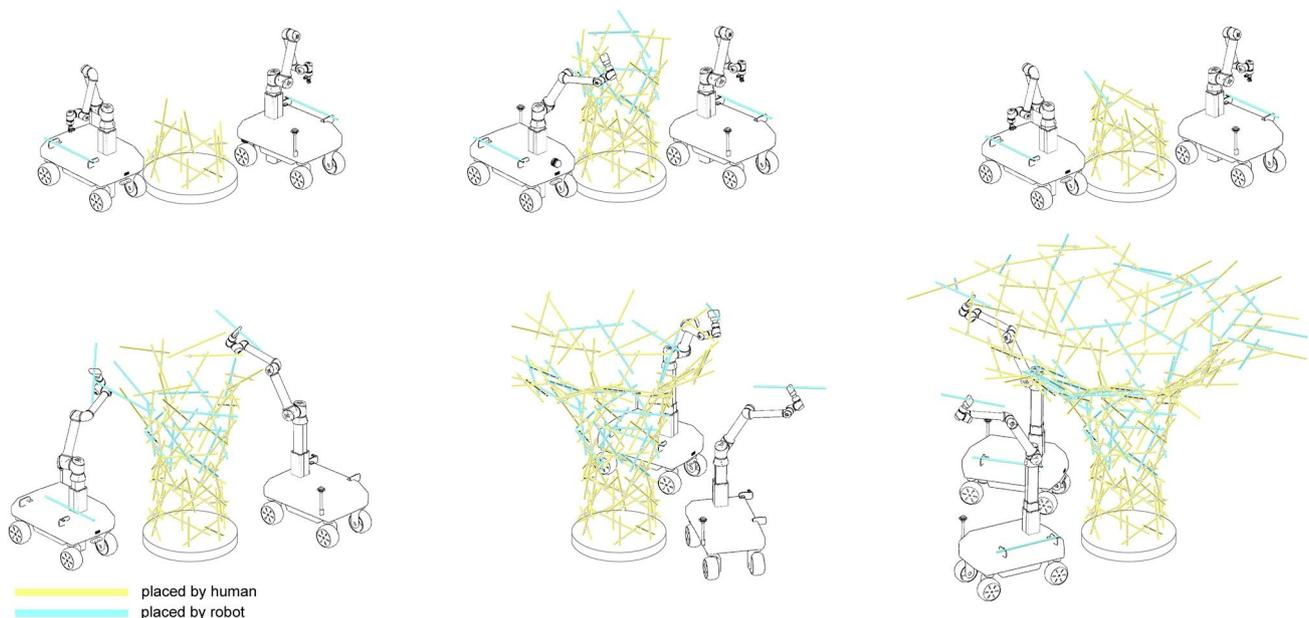
**Fig. 26** Assembly sequence generated during the design phase, illustrating the planned task distribution between two mobile robots and human agents. Color coding indicates which agent is responsible for placing each element
