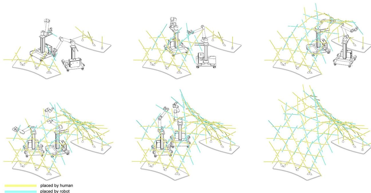
**Fig. 31** Assembly sequence generated during the design phase, illustrating the planned task distribution between two mobile robots and human agents. Color coding indicates which agent is responsible for placing each element
