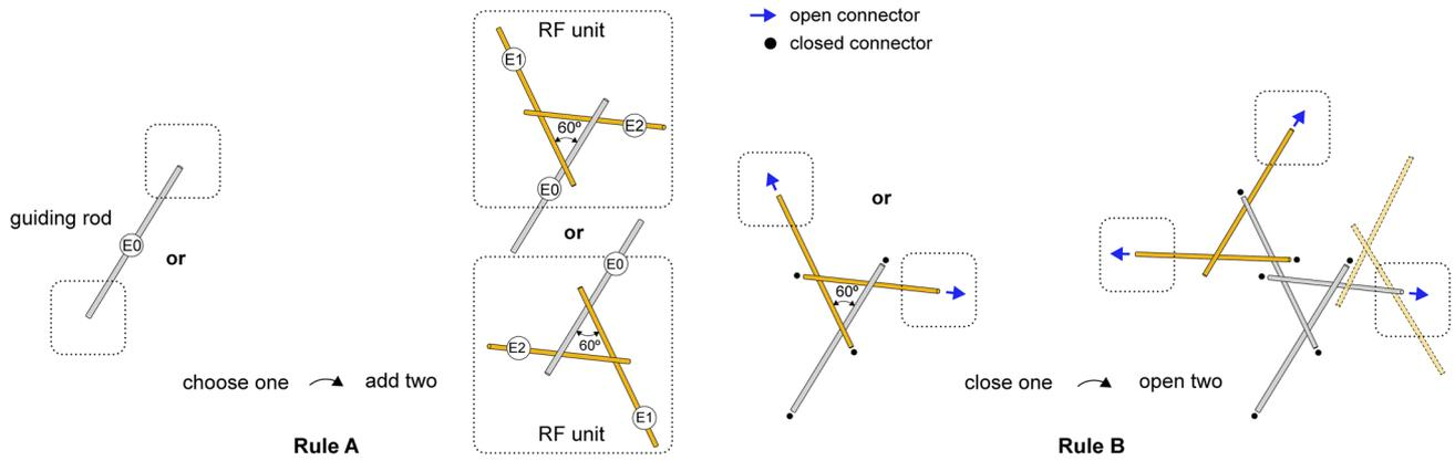
**Fig. 5** The primary rules of the assembly grammar: **Rule A**—formation of RF units via overlapping rods by attaching two rods to an existing guiding; **Rule B**—structural expansion via open connectors
