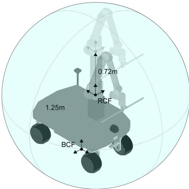
**Fig. 10** Robot reachability approximation: a sphere with a 1.3 m radius represents the robot arm's range, combined with a 0.72 m vertical extension enabled by the mobile system's linear axis
