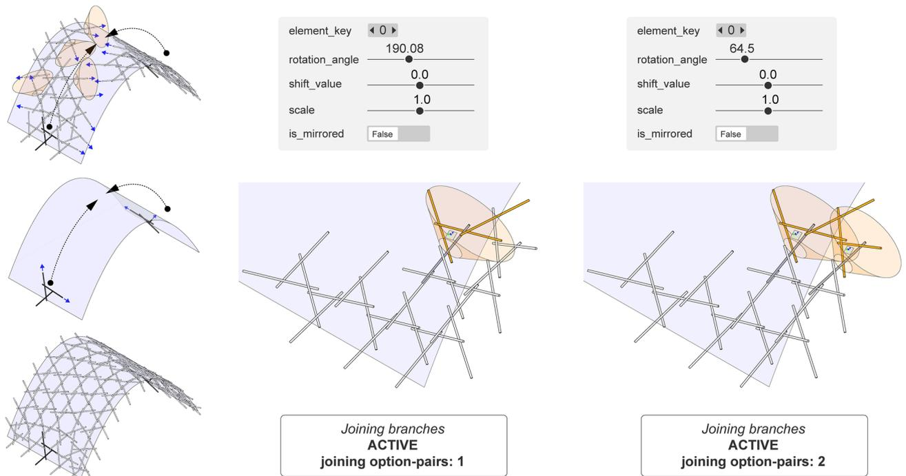
Fig. 8 Branching constraints: Multiple branches and open loops are generated when growing from multiple locations. These can be closed by identifying intersections between the ruled surfaces of open connectors, determined by the rod arrangements within modules
