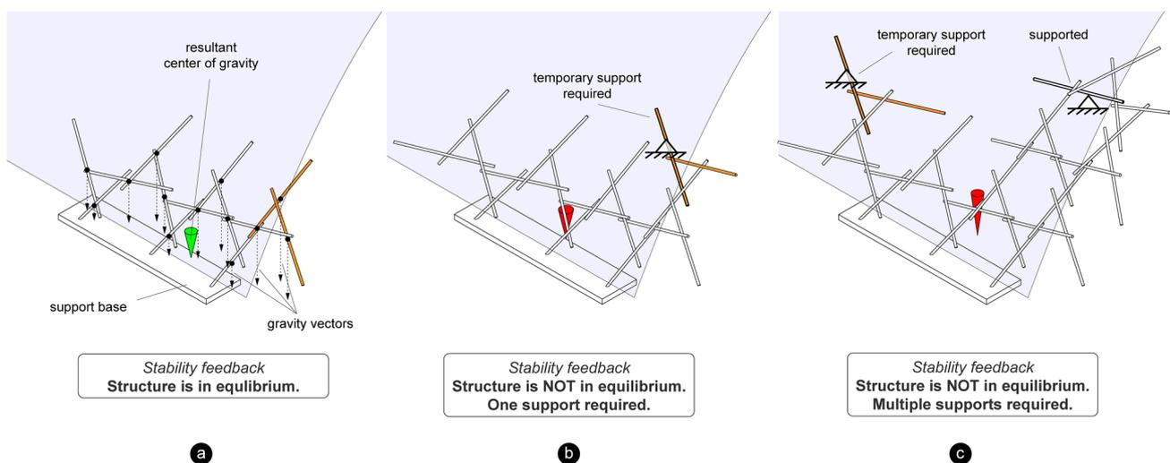
**Fig. 9** Equilibrium condition: stability is determined by verifying whether the resultant center of gravity, accounting for all elements of the branch in the current fabrication state along with the support base, falls within the support base’s footprint
