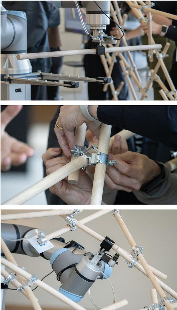
**Fig. 32** Humans and robots share the task of placing rods and supporting each other in their specific roles
