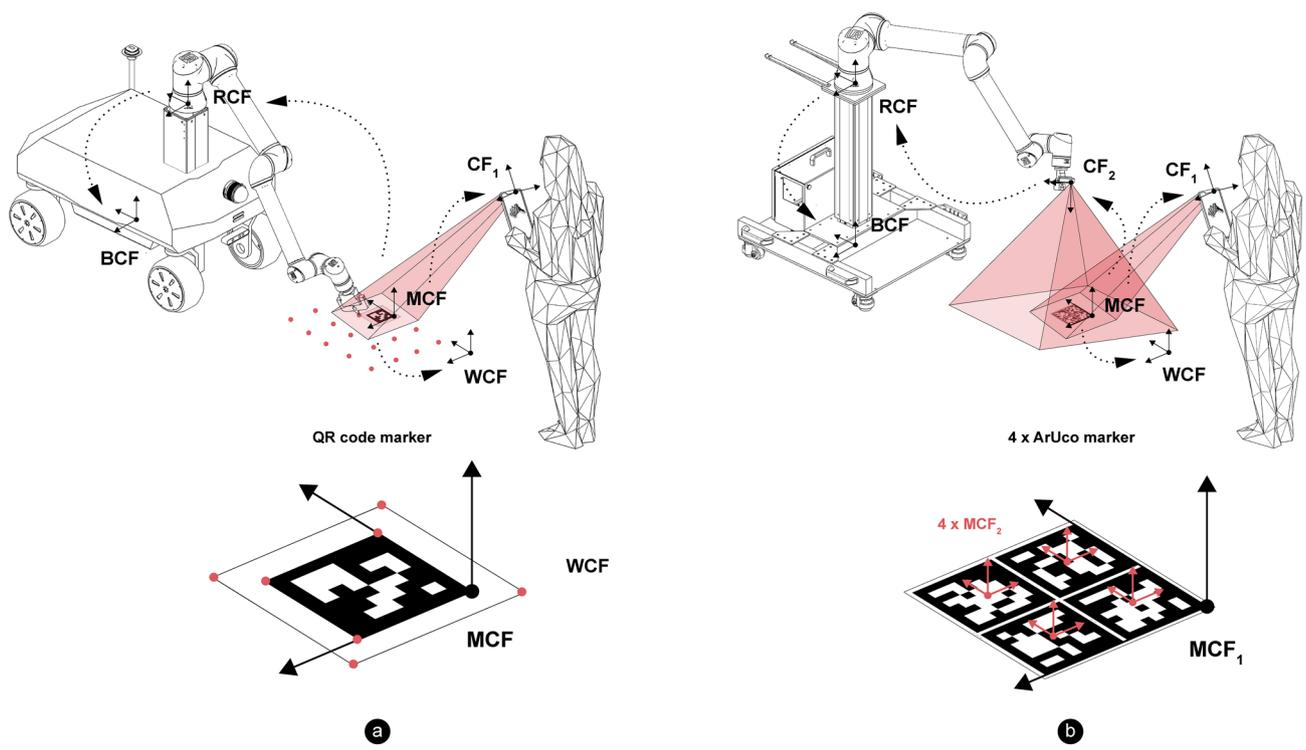
**WCF** - world coordinate frame      **RCF** - robot coordinate frame      **CF<sub>1</sub>** - phone camera frame
