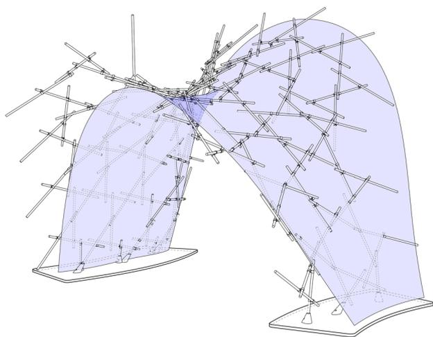
**Fig. 30** Final design of the timber demonstrator, including a visualization of the target geometry
