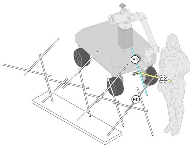
**Fig. 11** Human-robot task assignment: The guiding rod (E0) is pre-assembled first. The robot then places and holds the second rod (E1) steady until the human adds the third rod (E2), completing the RF unit
