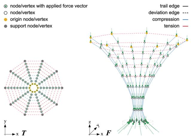
Fig. 24 Form-finding of the target geometry using CEM: the topology diagram ( $T$ ) defines connectivity, while the form diagram ( $F$ ) represents the equilibrium geometry. Curvature is controlled by adjusting trail lengths and internal forces in deviation edges
