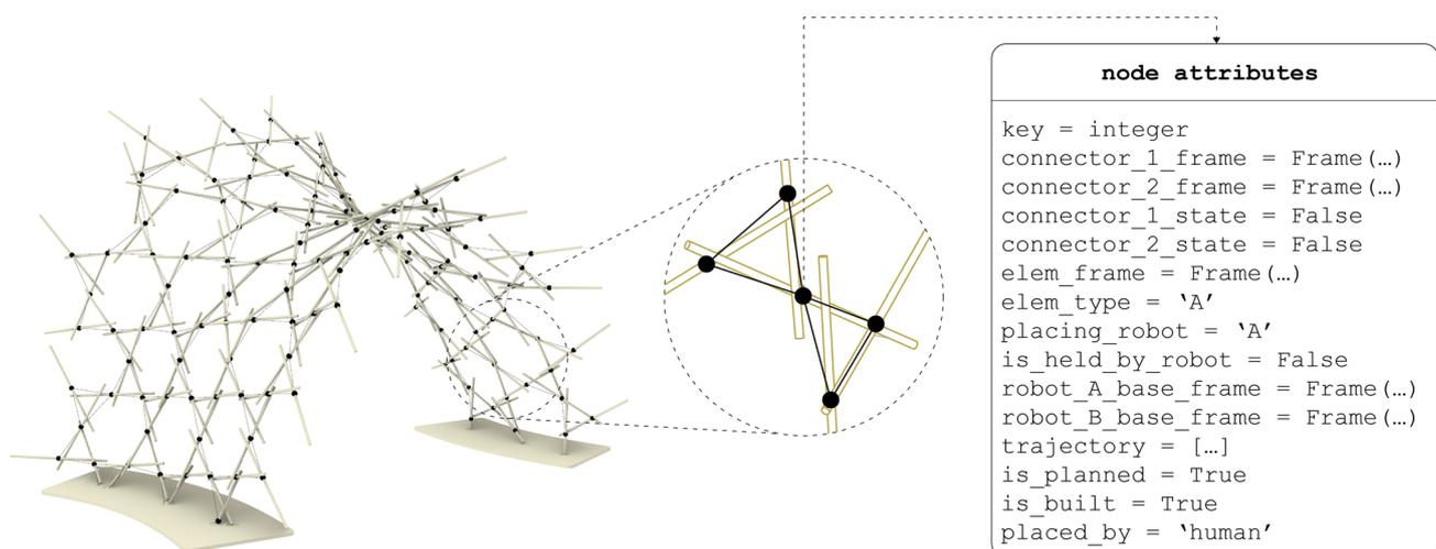
**Fig. 2** The AM is stored as a graph data structure, containing geometric and topological information of the architectural design model, connectivity between building elements, and design and fabrication attributes accounting for human–robot task distribution
