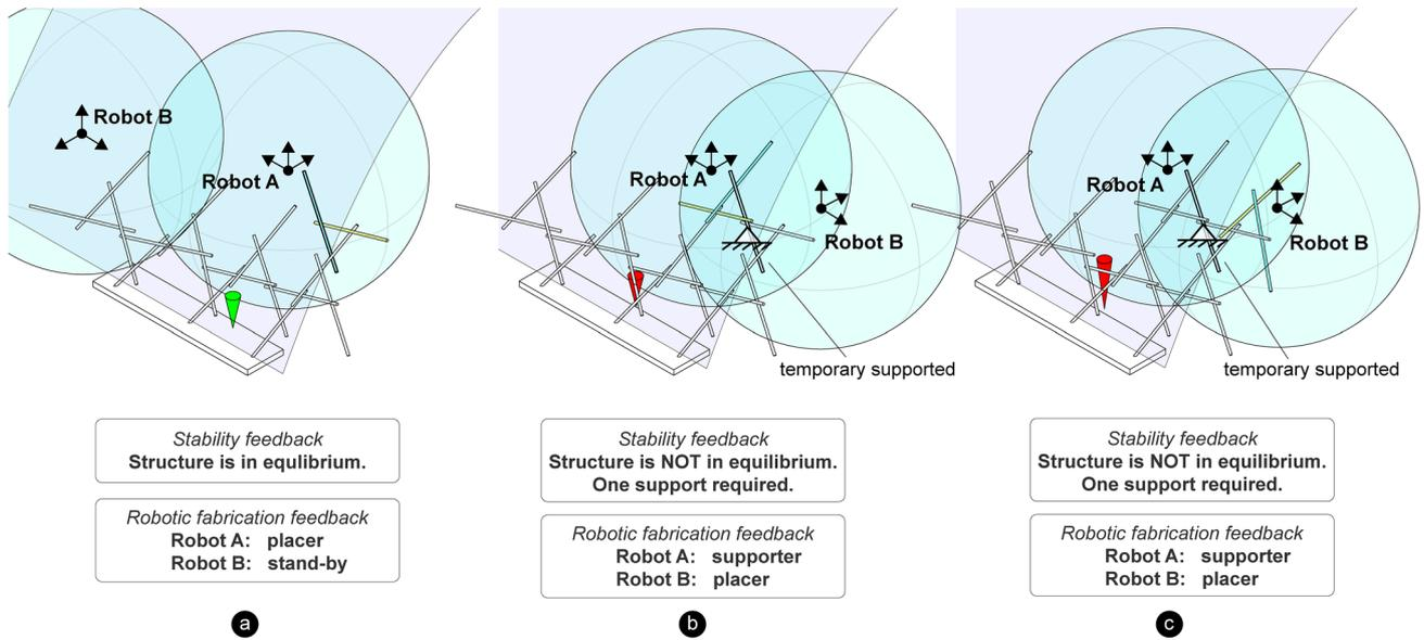
Fig. 12 Robot task assignment: Tasks are allocated based on availability and reachability, with the robots alternating between placer and supporter roles
