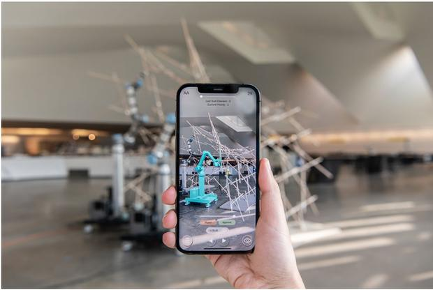
**Fig. 18** The custom AR phone-based application serves as a communication interface between the cooperating agents—human and robots—in the assembly process
