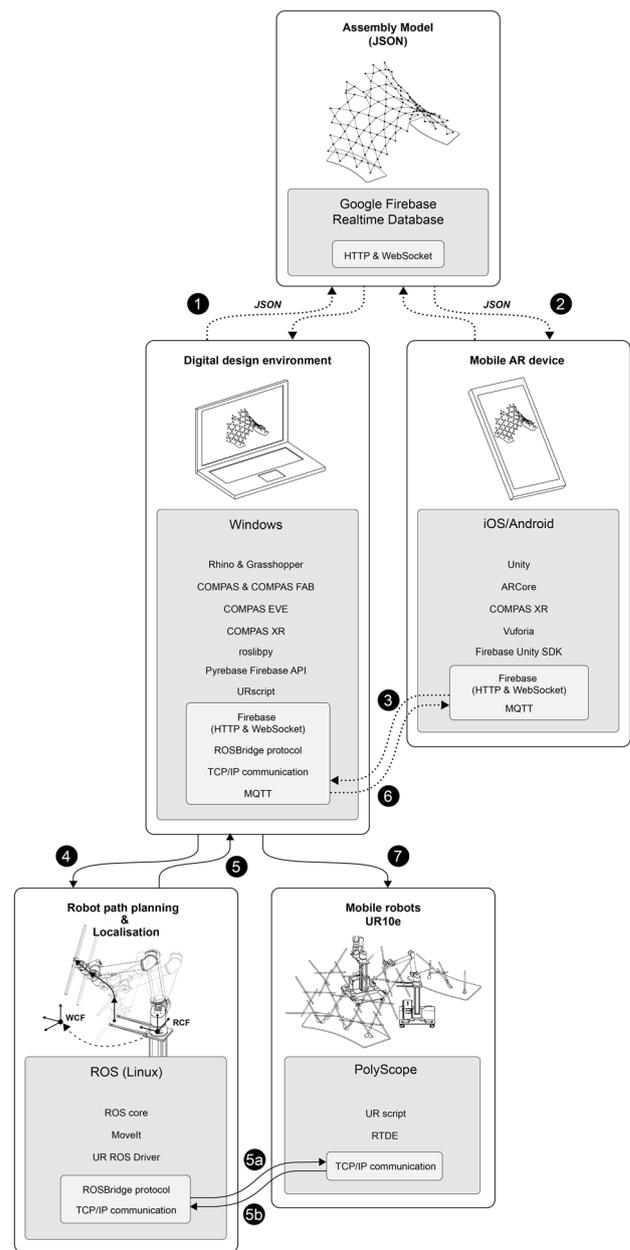
**Fig. 17** System backend architecture illustrating communication and data flow between digital design environment, cloud-hosted AM, robotic planning and simulation environment, and robot controller
