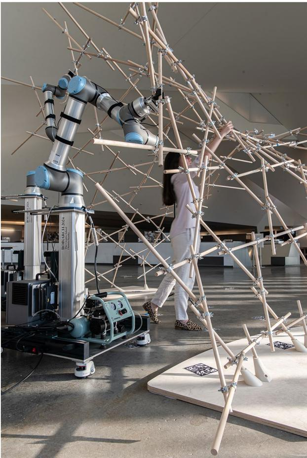
**Fig. 1** Human–multi-robot cooperative assembly of a timber structure
