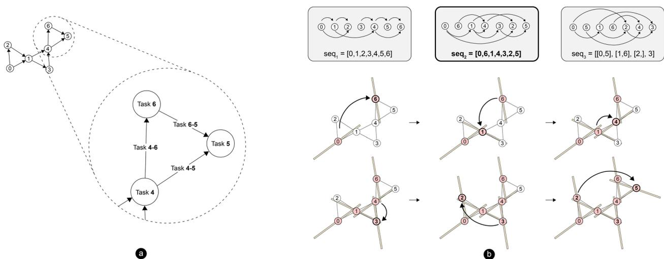
**Fig. 3** Task representation and sequencing: **a** The graph represents placement tasks through both nodes and edges, where the edge direction encodes dependencies between tasks. **b** The graph’s topology enables the generation of multiple valid task sequences
