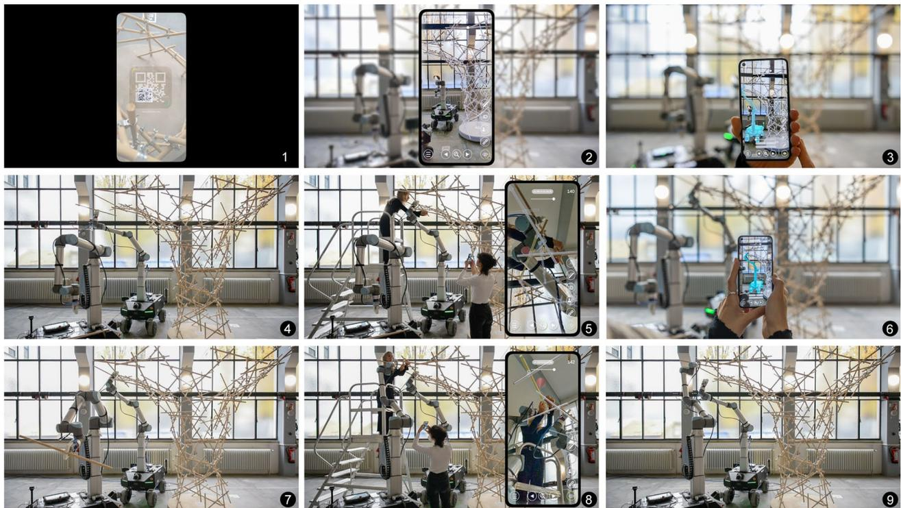
**Fig. 21** Steps of the cooperative assembly workflow involving a human–robot team consisting of two people and two collaborative mobile robots: (1) initialize the app, (2) visualize the geometry with the next element highlighted, (3) request the placement trajectory, (4) execute robotic placement with the assigned robot, (5) human places
