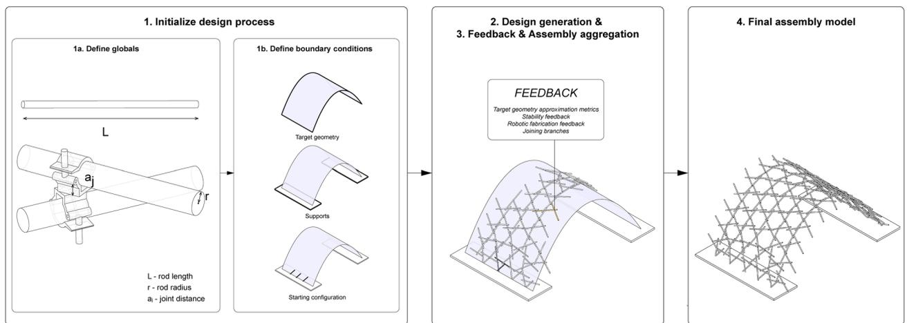
Fig. 14 The design process starts by defining the (1) boundary conditions of the intended design: these include the (1a) assembly globals and (1b) goal condition represented by the target surface geometry,
