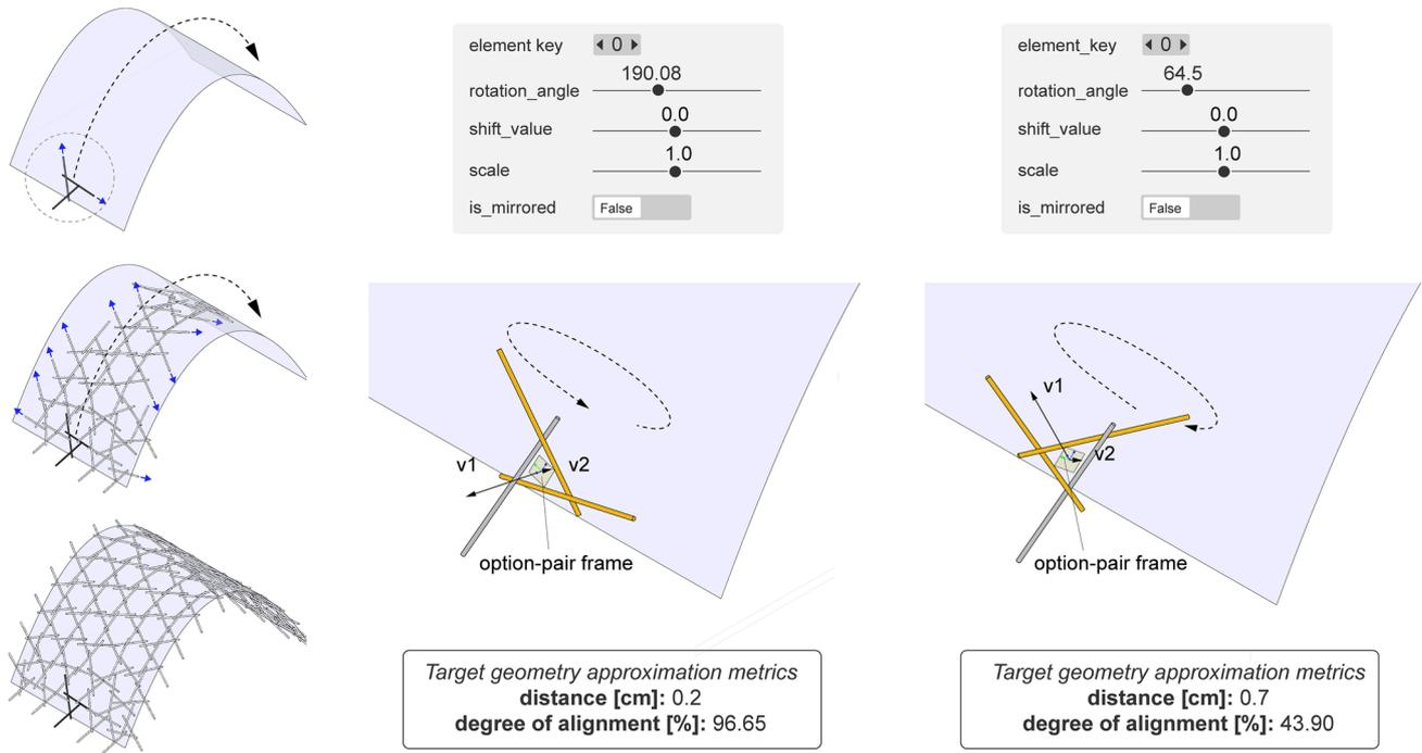
Fig. 7 Target geometry constraint: adjusting unit parameters based on distance and degree of alignment to conform to a predefined geometry
