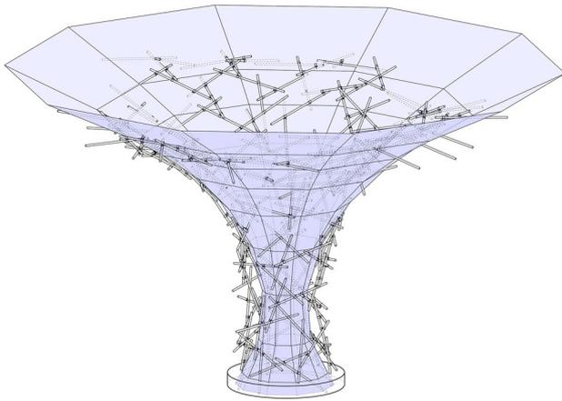
**Fig. 25** Final design of the timber demonstrator, including a visualization of the target funnel-shaped geometry
