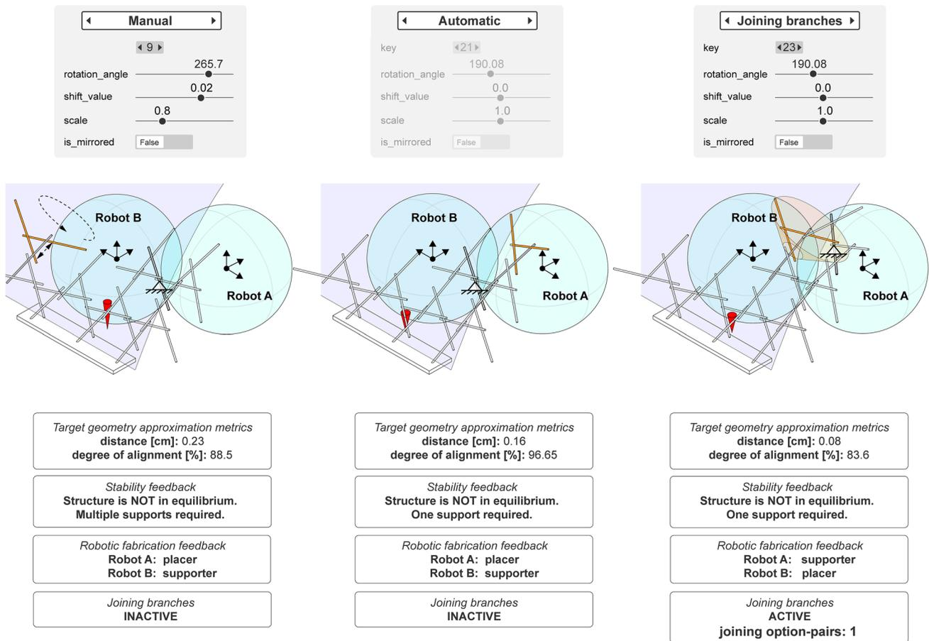
**Fig. 15** Three modes of design generation: manual, automatic, and branch joining
