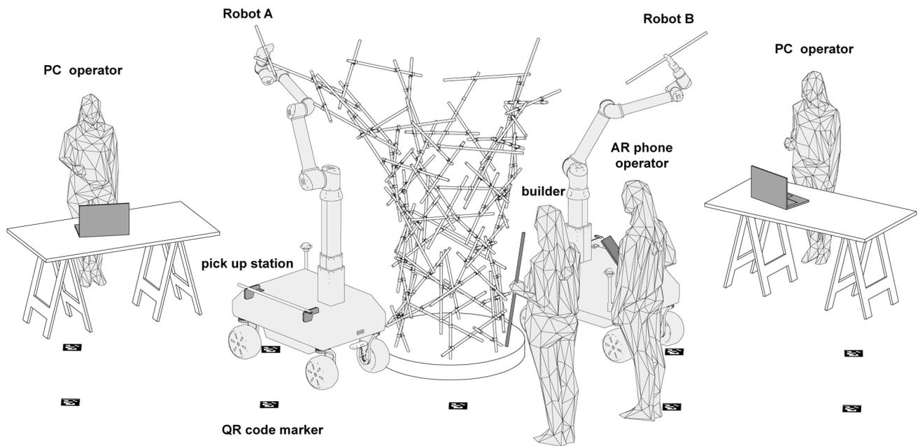
Fig. 23 Experimental setup of the cooperative assembly workflow for Case Study 1
