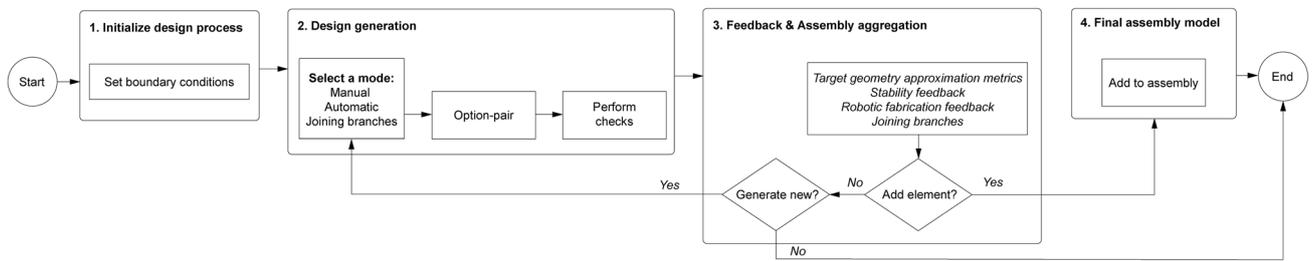
Fig. 13 Overview of the fabrication-aware computational design workflow, illustrating the key steps: (1) initialize design process, (2) design generation, (3) feedback and assembly growth, and (4) final AM
