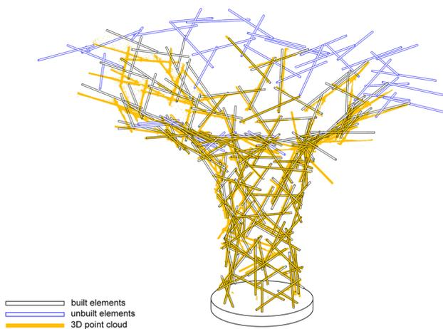
Fig. 27 3D laser scan of the partially assembled structure
