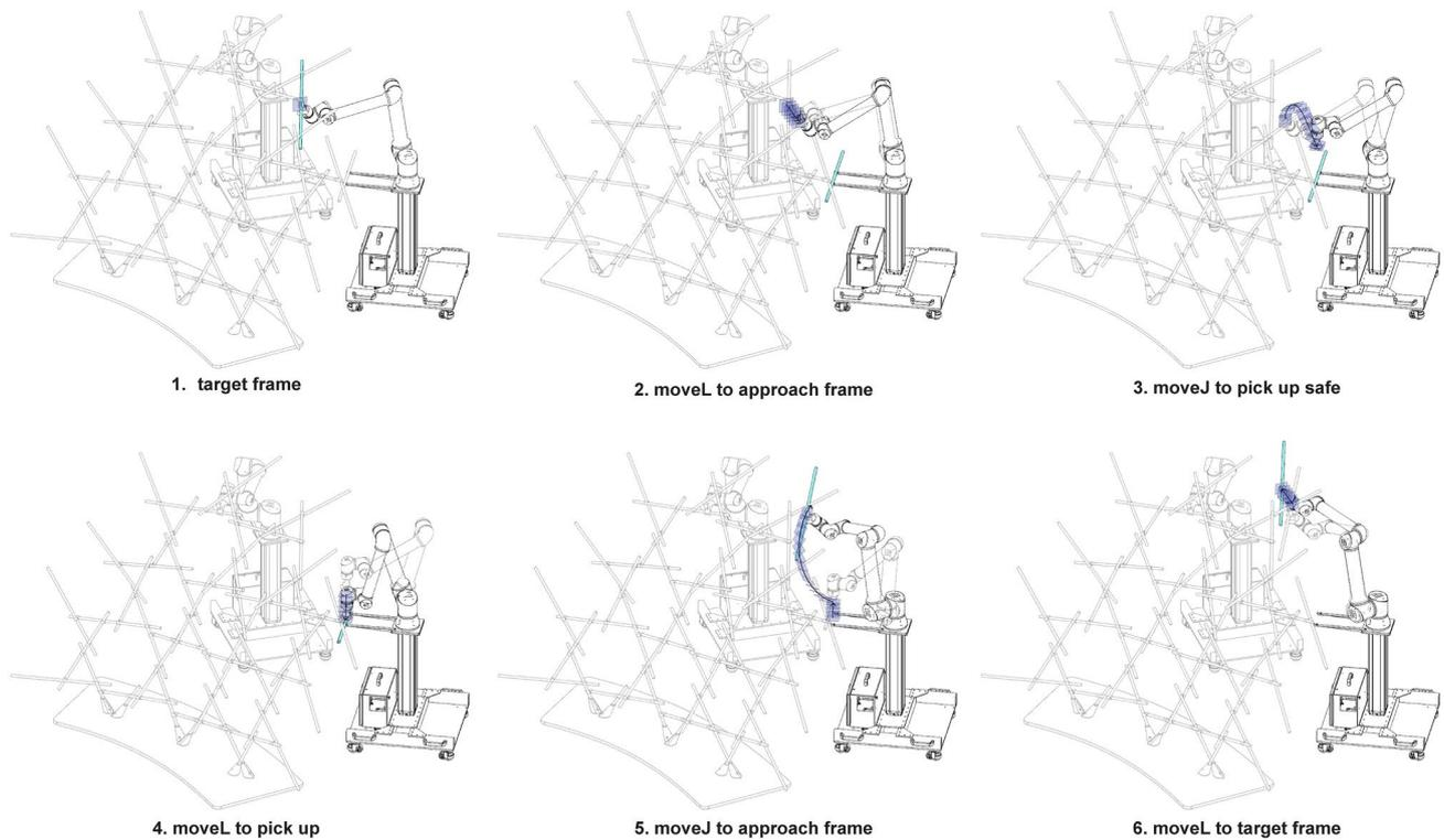
**Fig. 20** Robot motion planning: In-process computation of robot trajectories based on updated positions after mobile robot repositioning
