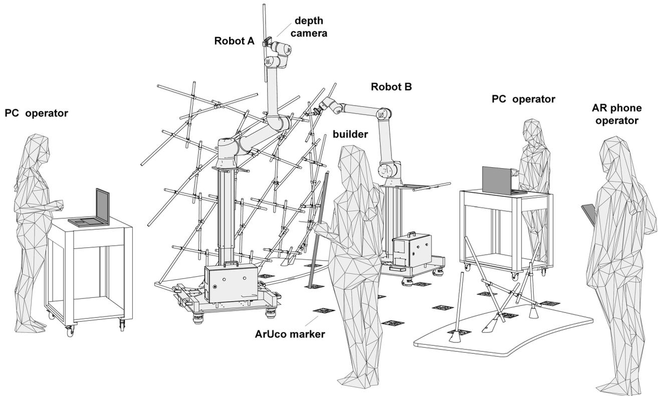
**Fig. 29** Experimental setup of the cooperative assembly workflow for Case Study 2
