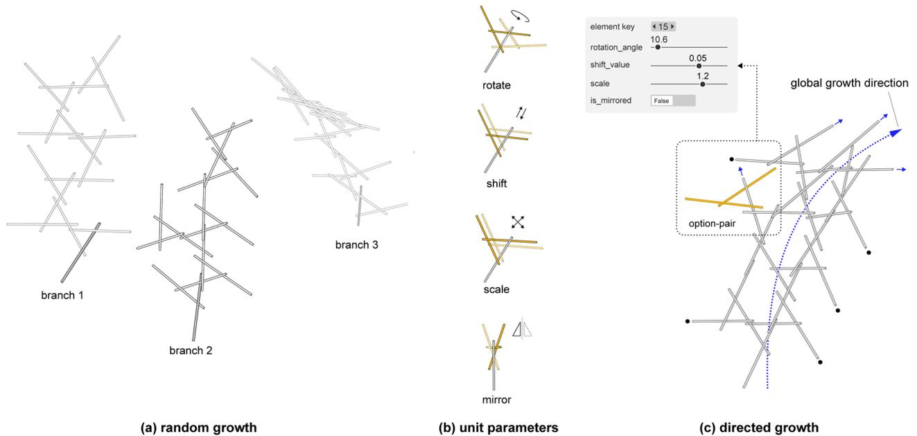
**Fig. 6** Assembly grammar growth: **a** random growth and branching behavior: When expanding a structure from multiple starting points, each guiding rod acts as the root of an individual branch. **b** By intro-
