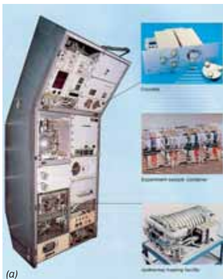
Figure 4.1.3. (a) The Materials-Science Double Rack (MSDR), flown on the first Spacelab flight and again on the German D-1 and D-2 missions. It contained two furnaces and several instruments supplied by Germany. France provided a furnace and Italy a Fluid-Physics Module. (b) ESA astronaut Ulf Merbold pictured working at the MSDR facility (courtesy of MBB/DASA)
