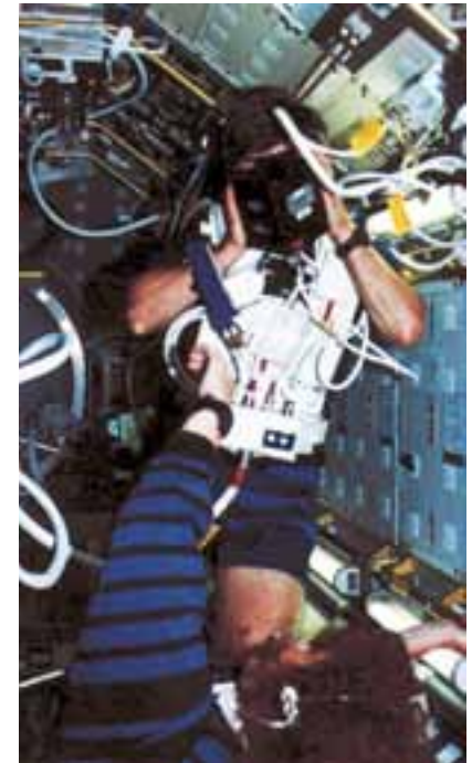
Figure 2.1.6.15. A free-floating crew member on the STS-78 mission, wearing a head-mounted visual stimulator and a vest carrying the 'Pocket' multi-channel portable recording system for measuring eye movement and muscle activity
