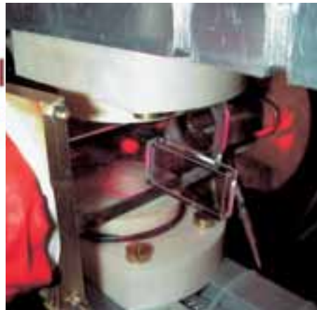
(b) A magneto-optical trap. In this glass cell, the red ball at centre is the fluorescence of a billion atoms, cooled and trapped by six laser beams. The two white rings hold the magnetic-field coils
