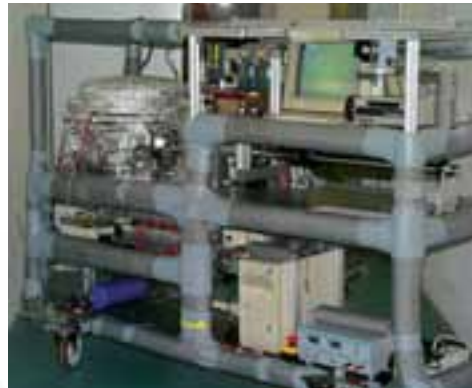
Figure 2.3.6.9. Equipment for metallic foam formation used on parabolic flights (courtesy of the Fraunhofer Institute, Bremen, Germany)
