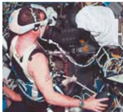
Figure 2.1.6.12. A crew member on the Neurolab STS-90 mission wearing the Virtual Environment Generator (VEG) head-mounted display. This display generated scenes that tested how the crew member maintained orientation in space
