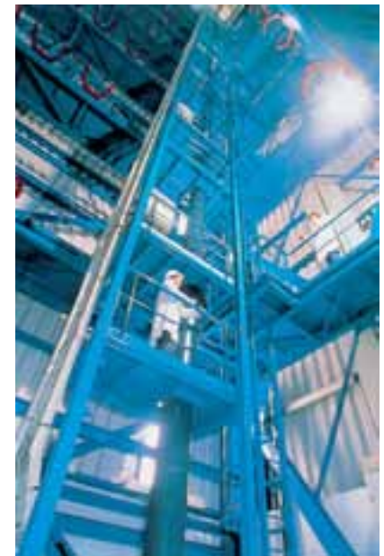
Figure 6.6.3. The drop tube in Grenoble (F), which provides 3 sec of weightless, free-fall conditions for solidification experiments (courtesy of CENG-Grenoble)
