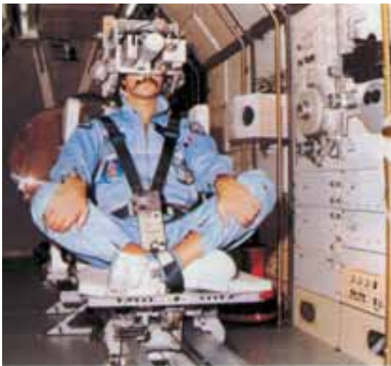
Figure 2.1.6.4. The ESA Space Sled, used on the German D-1 Spacelab mission. Providing linear accelerations along all body axes, it was used to evaluate possible changes in the detection threshold for very low linear accelerations in space
