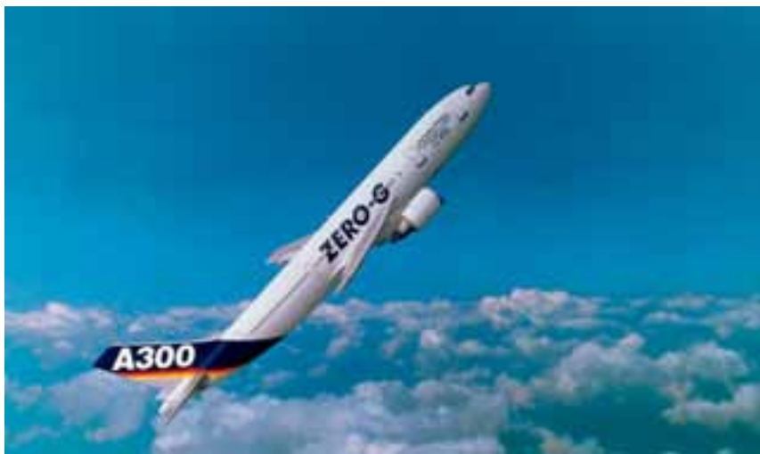
Figure 6.6.2. The Airbus A300 during a parabolic-flight manoeuvre, which creates low-gravity conditions lasting about 20 seconds (courtesy of Novespace)
