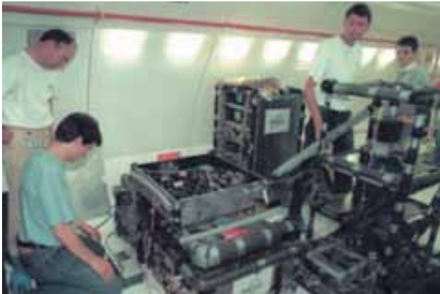
Figure 2.3.10.8. The PHARAO prototype under test on the CNES Zero-G Airbus in 1997
