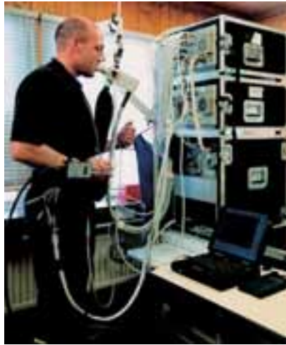
Figure 6.4.2. The Respiratory Monitoring System, used on the 179-day Euromir '95 mission to monitor the cardiovascular system and pulmonary performance
