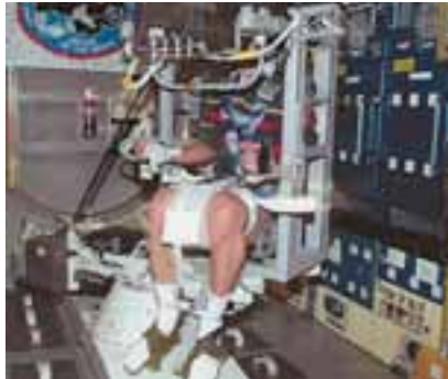
Figure 2.1.6.9. The ESA Visual-Vestibular Integration System, or off-axis rotator, used on the Neurolab STS-90 mission. In space, this short-arm centrifuge stimulated the vestibular system through a 0.5g or 1g linear acceleration directed along the subject's inter-aural axis, without the confounding effect of gravitational acceleration
