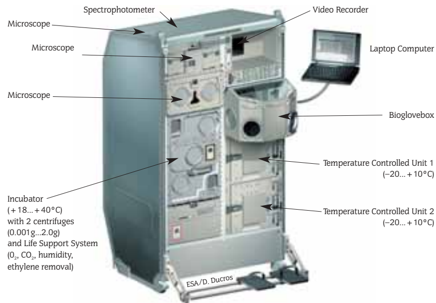
Figure 5.2.2. The ESA 'Biolab' multi-user facility for biological research. The loading of samples and operations in the Bioglovebox are conducted by a crew member. Thereafter, the experiments are performed automatically, with the possibility of remote guidance/intervention from a ground-based scientist
