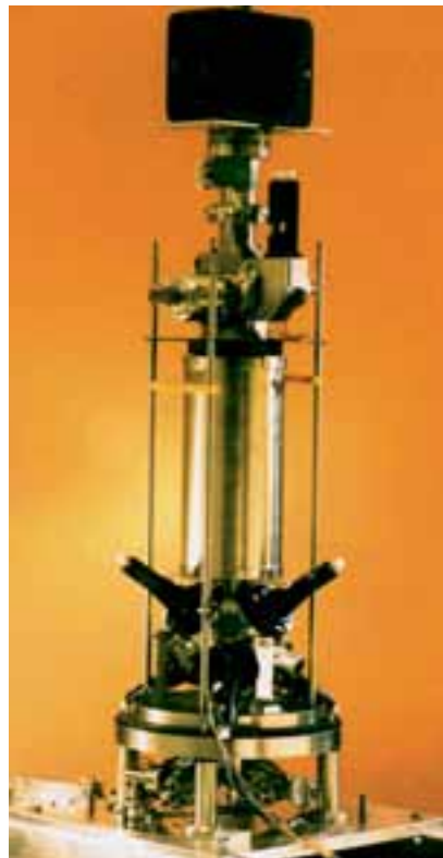
Figure 2.3.10.9. The PHARAO caesium tube (total length 1 m). Bottom: cooling zone. Middle: interaction zone. Top: detection zone and vacuum pump
