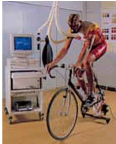
Figure 3.2.5. The Innovision Respired Gas Analyser. Derived from a space instrument for ESA, it provides a non-invasive method of determining cardiac output and lung characteristics and functions (courtesy of Innovision)
