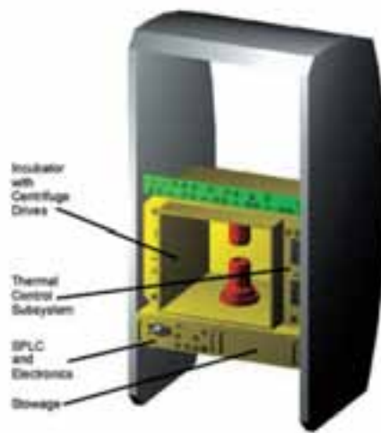
Figure 5.2.9. The European Modular Cultivation System (courtesy of Astrium/DASA)
