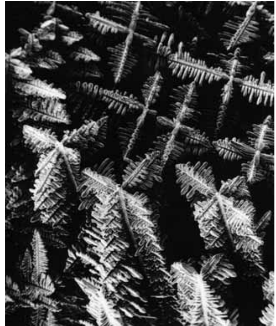
Figure 2.3.3.5. Columnar dendritic growth in a directionally solidified Co–Sm–Cu peritectic alloy. The view of the dendrite array is obtained by etching away the Co_{17}Sm_2 matrix from the primary Co dendrites (courtesy of R. Gardon & W. Kurz, EPFL)
