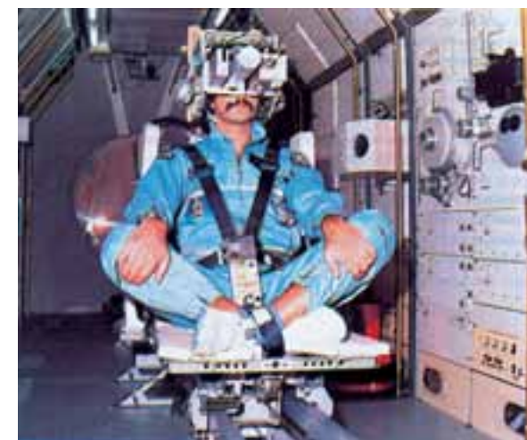
Figure 4.1.4. ESA astronaut Wubbo Ockels testing the Vestibular Sled, used to study motion and orientation perception in weightlessness
