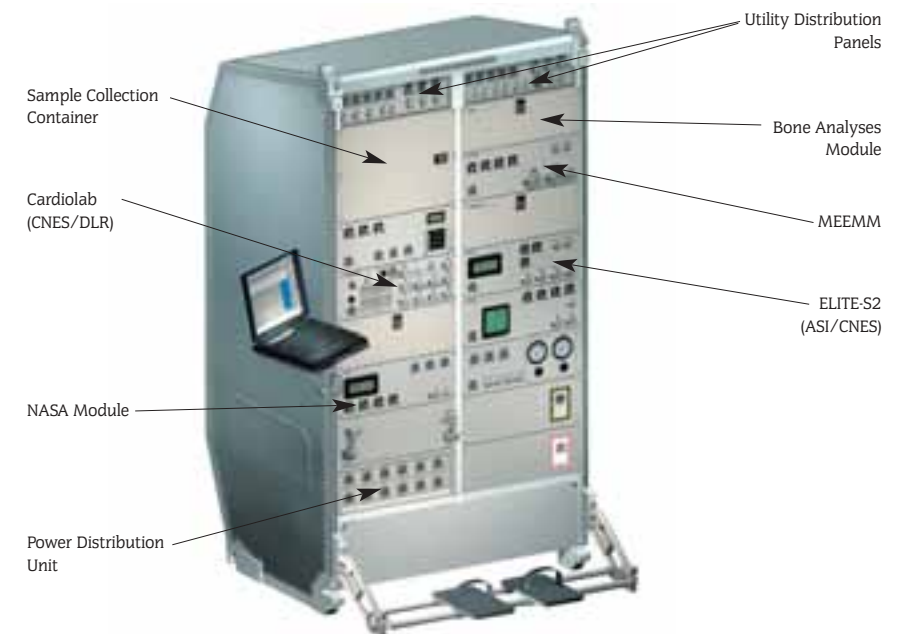
Figure 5.2.4. The European Physiology Modules, to be located in the ESA Columbus Laboratory. The NASA Human Research Facility will be co-located there to allow combined experimentation
