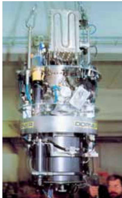
Figure 4.1.5. The German 'Tempus' Experiment Module. Electromagnetic levitation allows high-temperature reactive melts to be studied without having to use a container. An ESA follow-on development of this system will be used in the ISS/Columbus Materials Science Laboratory (courtesy of Astrium/Dornier)
