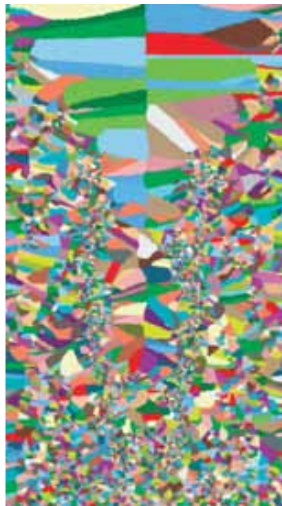
Figure 2.3.3.17. (a) Longitudinal cross-section of an aluminium-base alloy cast in a steel mould (120 mm high and 60 mm in diam.). A sedimentation cone of fine equiaxed crystals is clearly seen at the bottom of the ingot, as in Figures 2.3.3.1 and 2.3.3.7b, and a coarse columnar structure at the top (from N.L. Cupini et al., in 'Solidification and Casting of Metals', Metals Society, London, 1979, p. 193).
