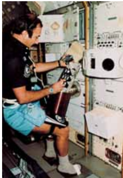
Figure 4.2.1. The ESA 'Biorack', which accommodated 14 cell and developmental biology experiments on the Spacelab D-1 mission and was later used on the two further Spacelab and three Spacehab missions. ESA astronaut Wubbo Ockels is seen here working at this facility
