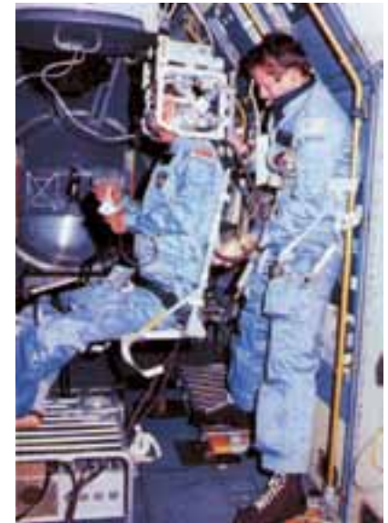
Figure 2.1.6.13. The first eye-movement recording system, with a video camera, developed by ESA for experiments during the first Spacelab mission
