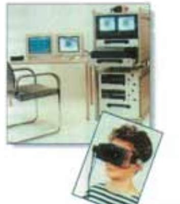
Figure 2.1.6.14. The Video-Oculography (VOG) Unit, developed by DLR for use on the ISS
