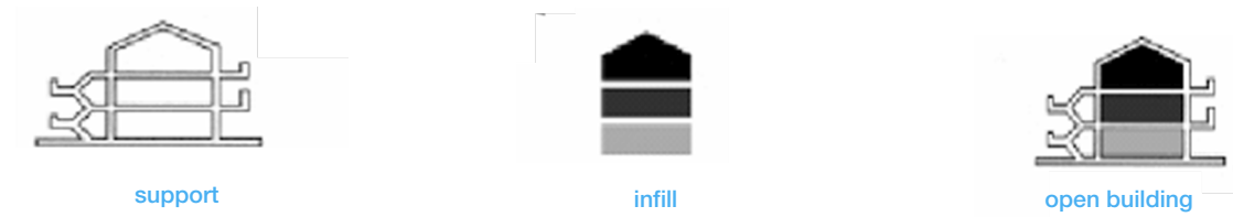
Figure 25: John Habraken's Open Building Theory of separating the support and infill. "Open building makes a distinction between support and infill. The support represents the most permanent part of the building, like the structure. The infill represents the adaptable part of the building." (Habraken, 2002)
