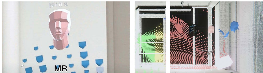
Fig. 6. Fabrication supervision feature. On the left is a first-person view of the MR-User looking at the VR-User. On the right side is a third-person camera view of the MR and VR-User discussing the fabrication in VR. The different colored elements show the different fabrication sessions.
