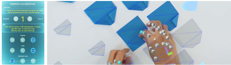
Fig. 5. A menu informing the MR-User about fabrication parameters and the holographic 3D model supporting fabrication.
