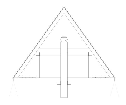
The dimensions are based on the size of the fish ball. The roof construction rests on the column. The fish ball is placed on the column under the ridge in the attic. Construction of a roof.
