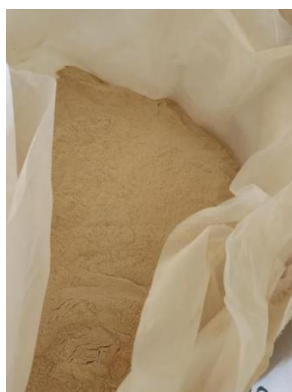
Fig 13 Jurisdictional Imaginary 4 . by 18% Taiwan Artocarpus treculianus flour PLA 3D printing filaments with silky texture
