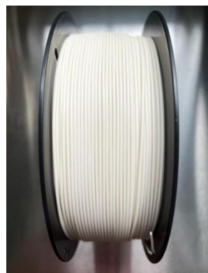
Fig 13 Jurisdictional Imaginary 4 . by 18% Taiwan Artocarpus treculianus flour PLA 3D printing filaments with silky texture
