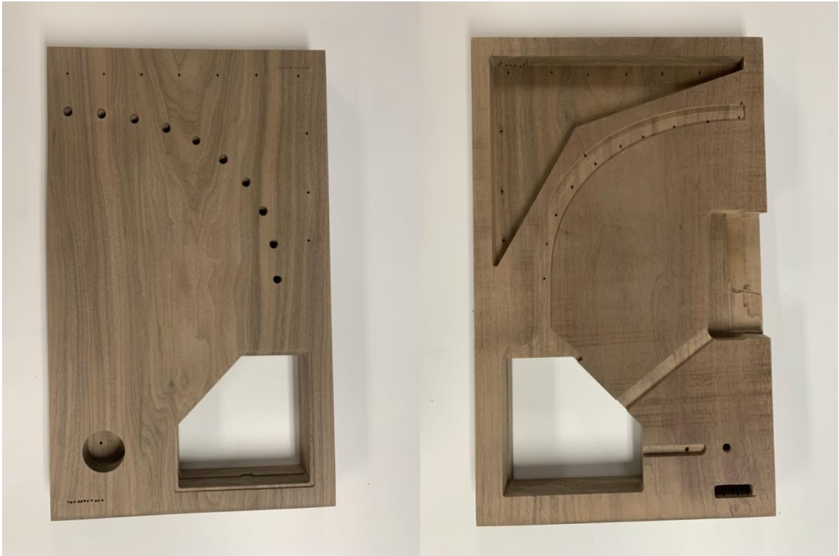
Fig. 16: The CNC cut walnut body from above (left) and below (right). The cuts underneath allow for wiring, tuning pegs, and jacks to be installed.
