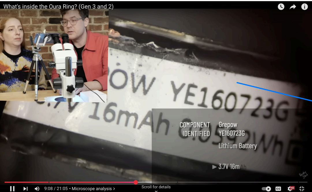
Lithium Battery 3.75V 16mAh
