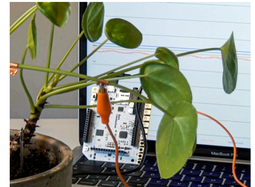
Figure 48 & 49: Capturing touch signals with Devil's Vine & Jade Plant in a graph using the program Processing.
