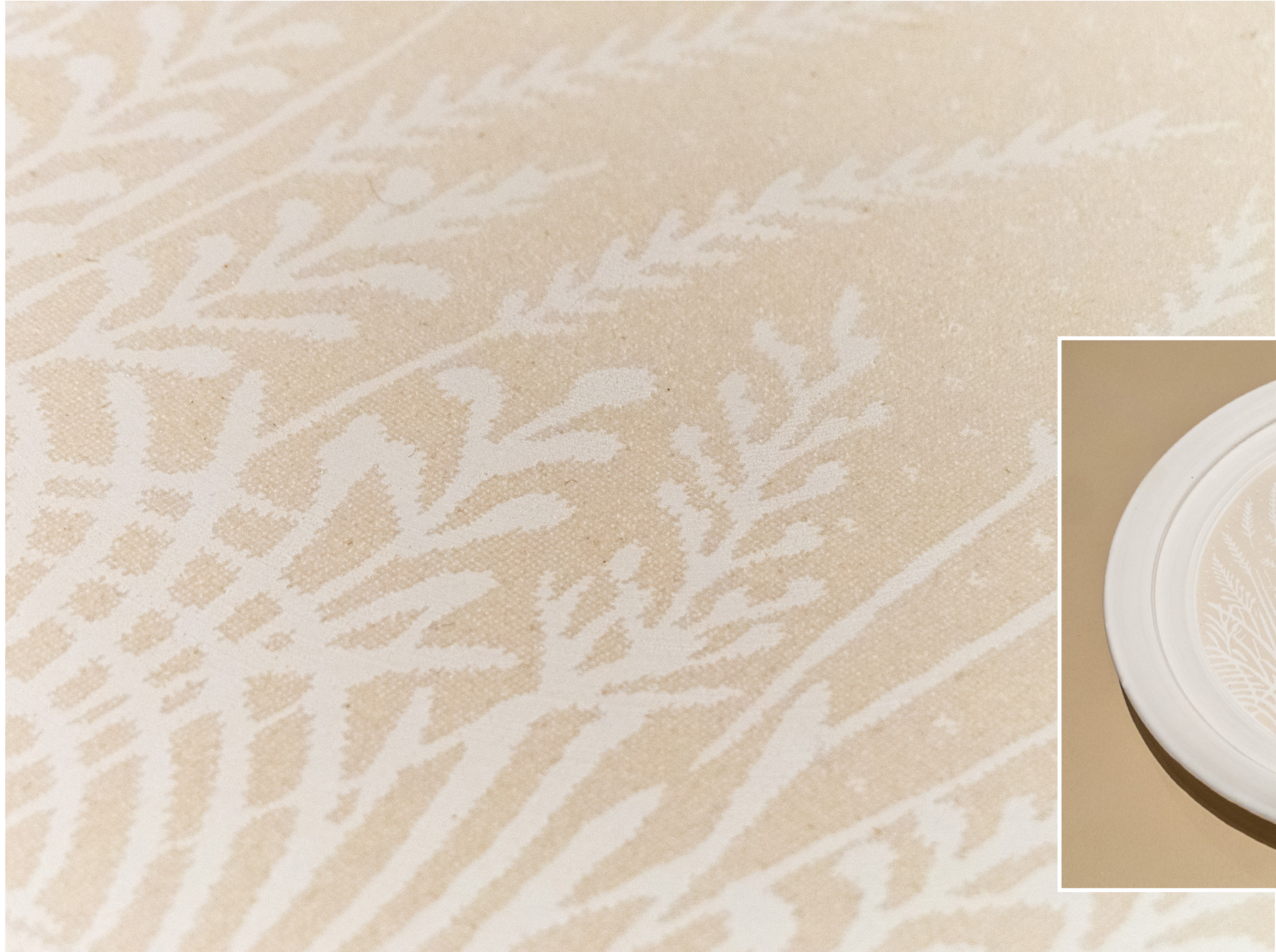
Plate 30 cm diameter Laser etching on porcelain (unglazed and unpigmented)
