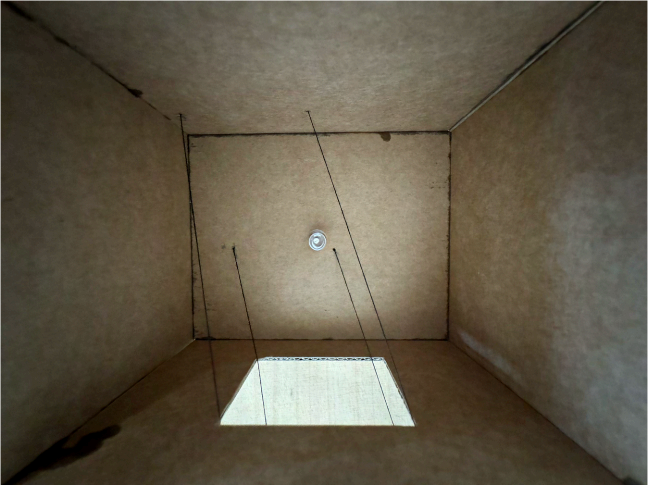
FIGURE 9 INTERNAL VIEW OF PILOT STUDY MODEL. BLACK THREAD FORMS THE BOUNDS OF THE 'SHAPE OF LIGHT'.
