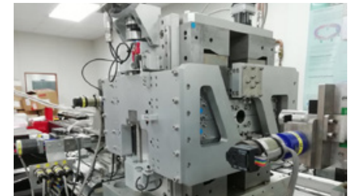
The Diamond Light Source ZEPTO quadrupole fully assembled and in position for testing
