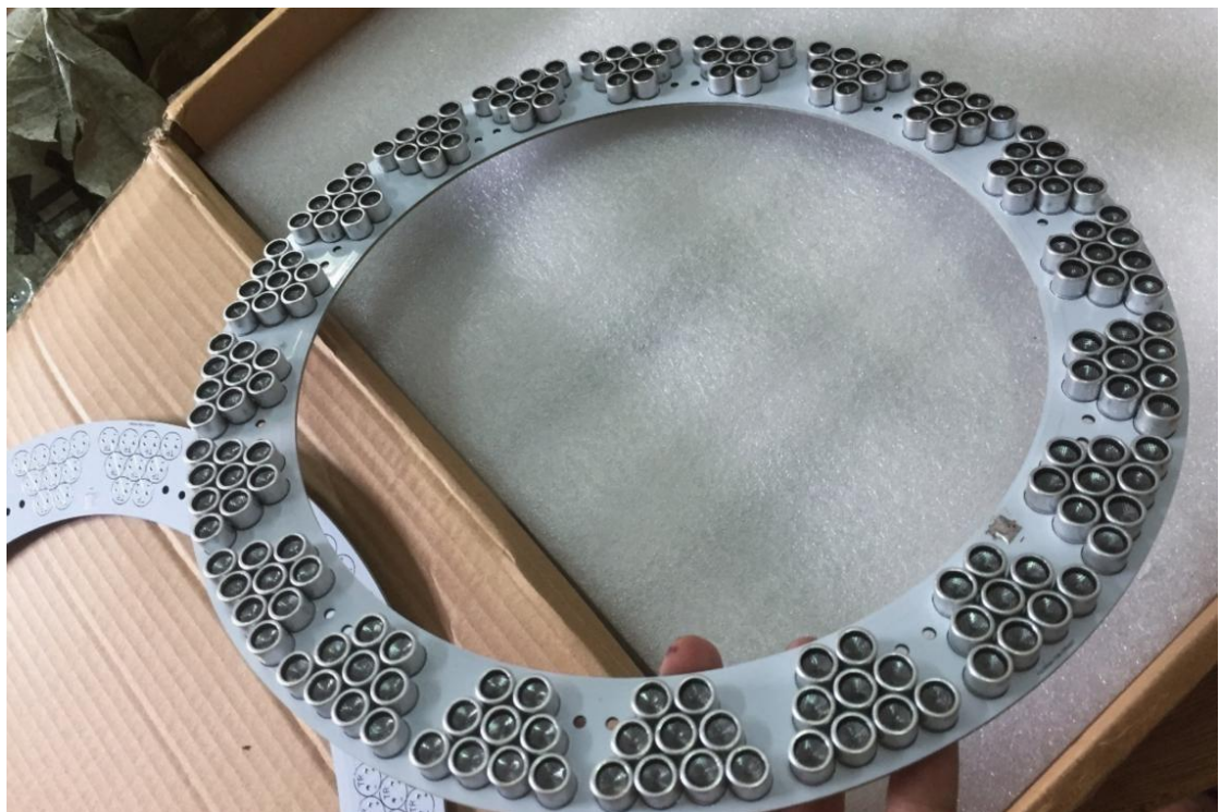
Whispers of Breeze (C-Lab), 2020 | an Ultrasonic Directional Speaker module specifically designed to match the size of the ceiling fan
