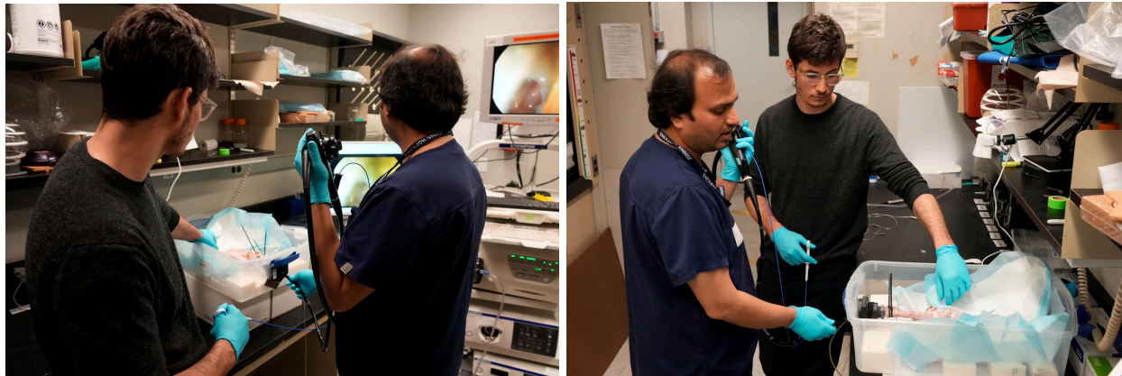
Figure 4: Device being deployed in a simulated GI tract (pig stomach)
