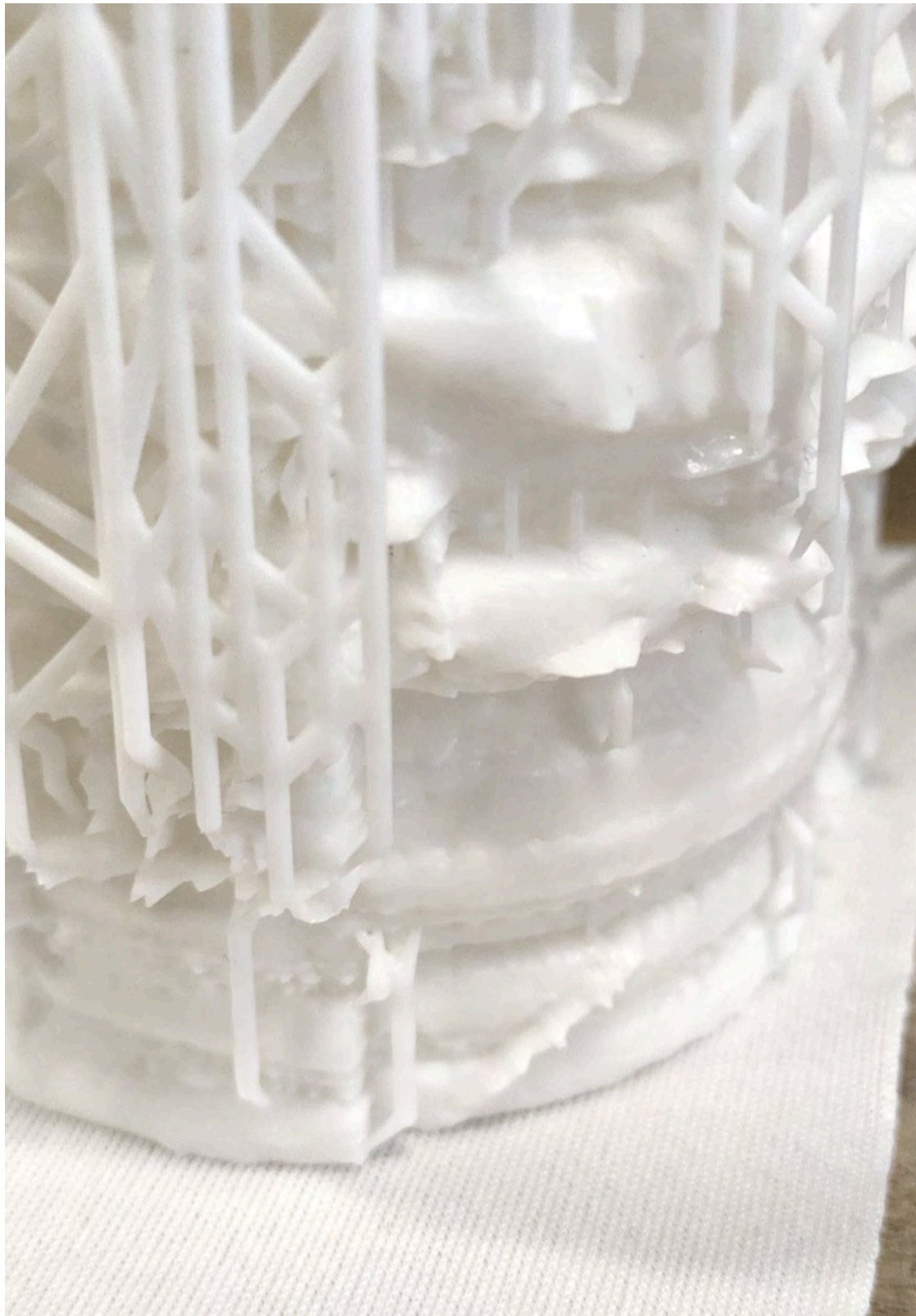
3d printed object with supports generated in the process of fabrication
