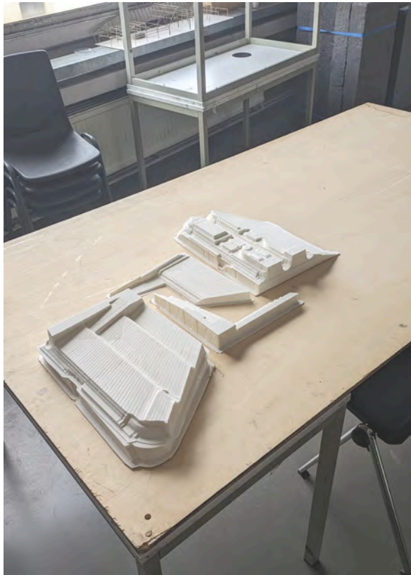
The pieces of this volume carved by the CNC are refined and assembled by hand using an exacto knife, sand-paper and glue
