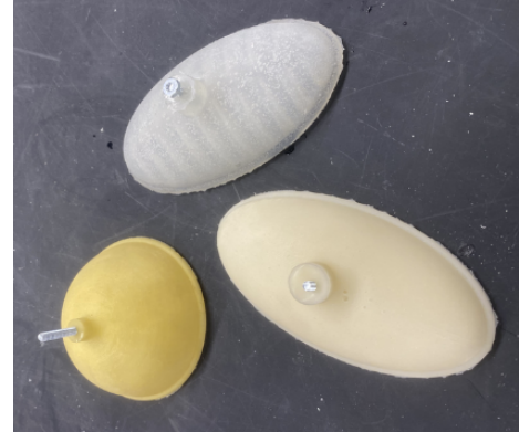
Fig. 2. Top: Ecoflex 00-31 Remora, Bottom Left: Vytaflex 60A Regular, Bottom Right: Vytaflex 40A Remora
