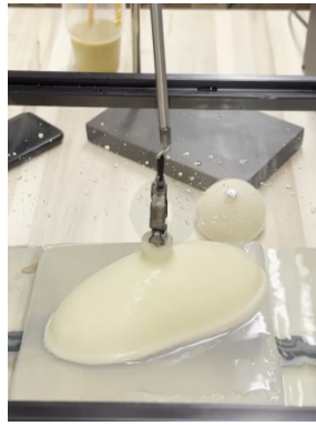
Fig. 4. Remora Suction Cup Apparatus in Wave Tank
