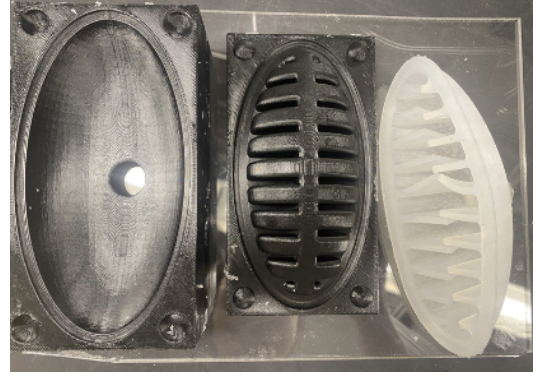
Fig. 1. 3D-Printed Mold and Remora Suction Molded with Ecoflex 00-31
