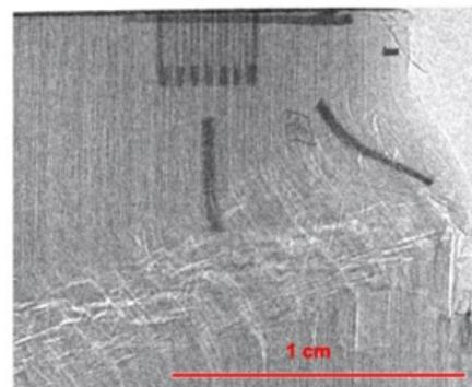
Radiograph of kink band failure in a composite material, obtained with the laser-betatron source. Individual carbon fibre tows are visible.<sup>3</sup>
