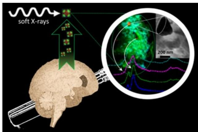
*Synchrotron soft X-ray nano-imaging and spectromicroscopy reveals iron and calcium biomineralization in Alzheimer’s disease amyloid plaques (Image: Diamond Light Source)*
