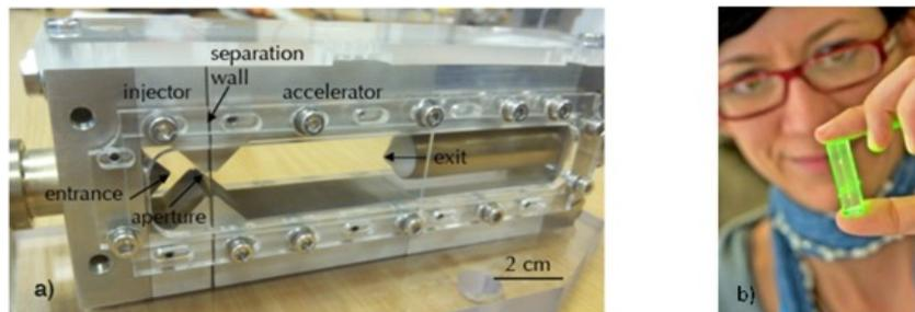
(a) and (b) Centimetre-scale plasma accelerators used in Gemini
