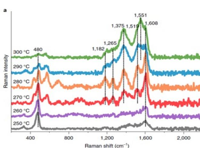
*The spectral “fingerprint” shows the build-up of contaminants as temperature increases*
