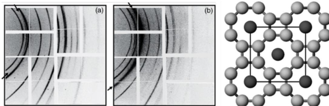
(Left) 2D diffraction images collected from the LCLS XFEL on a single CSPAD detector from (a) uncompressed (hcp) scandium and (b) scandium compressed to 51.1 GPa.
