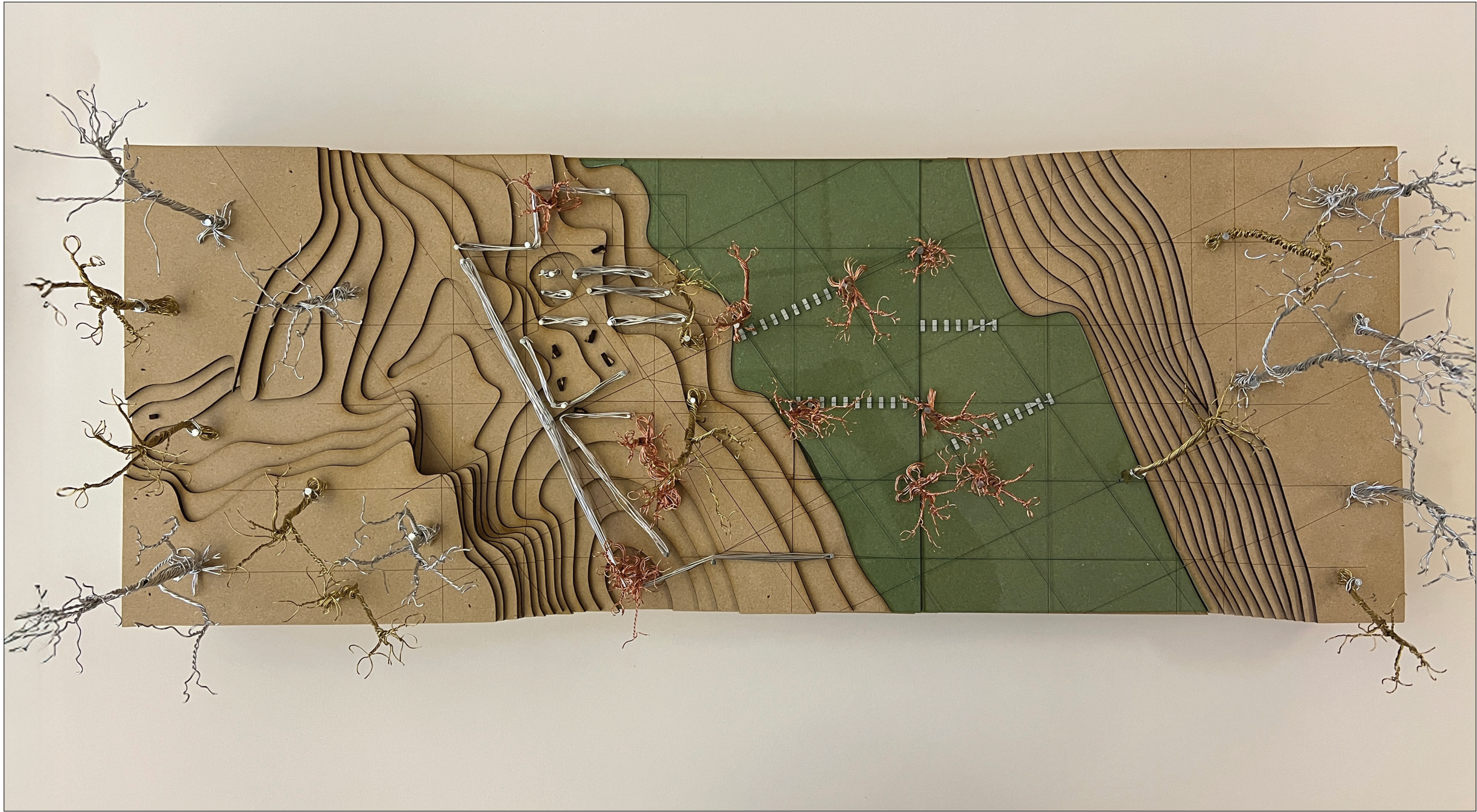
Site model made of stacked MDF, laser cut acrylic, twisted wire, and nails.
