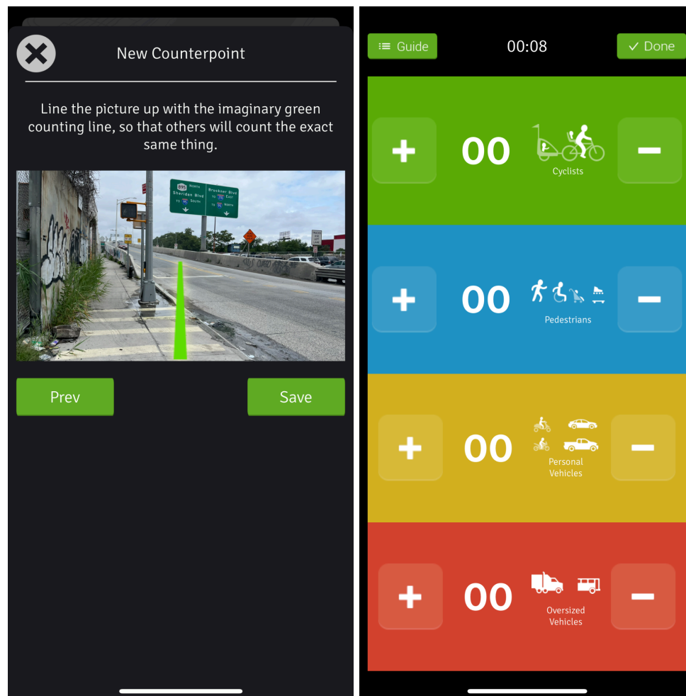
Figure 3. Using the CounterPoint application to create counting lines and count commercial vehicles.
