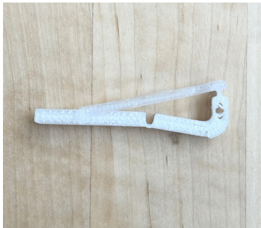
Figure 1.2 Increased the total length of the brace from 45mm to 52 mm.
