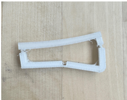
Figure 1.7 Pre 16.0. The hinge position is at the lower left and the prototype is not bistable.
