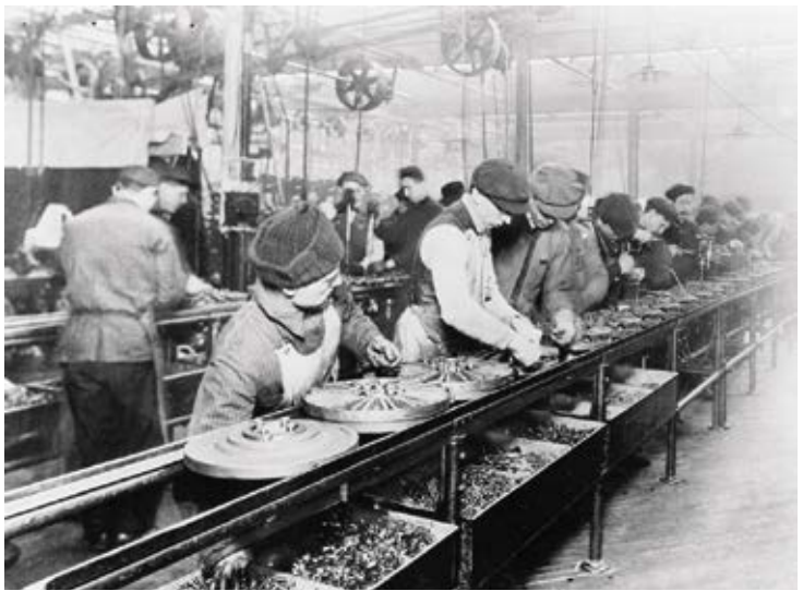
Ford workers on the first moving assembly line, Highland Park, MI, US, 1913.
