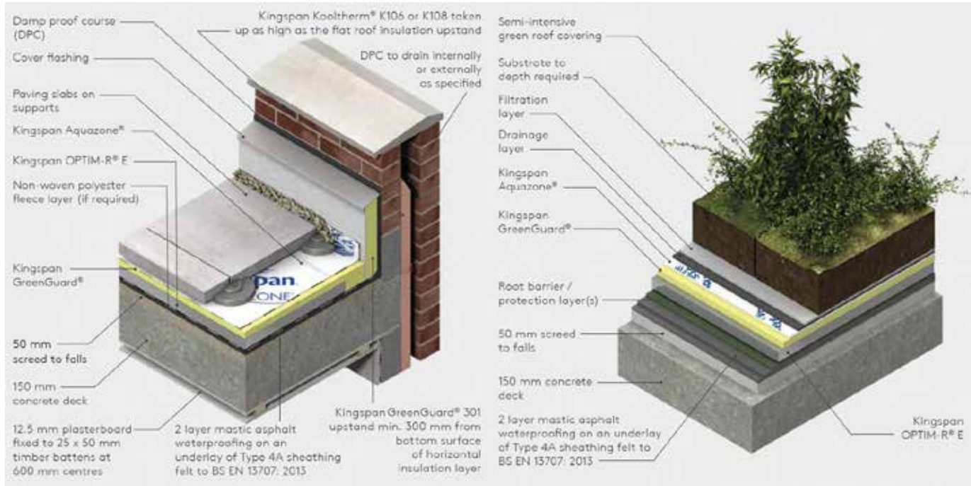
An inverted roof flips traditional roofing design by placing insulation on top of the waterproofing membrane. This setup protects the membrane from weather and UV rays, also working to extend the roof's overall life. The insulation maintains its effectiveness despite exposure to the elements. Above the insulation, a protective layer adds extra defense and improves the building's thermal efficiency. This system is then finished with paver stones, loose gravel, or green roofing. The inverted layout keeps the membrane at a more stable temperature, reducing the risk of damage due to thermal changes. When paired with green roofs, such as that in Odham's Walk, the insulation effects are enhanced as well as improving the building's overall environmental footprint.
