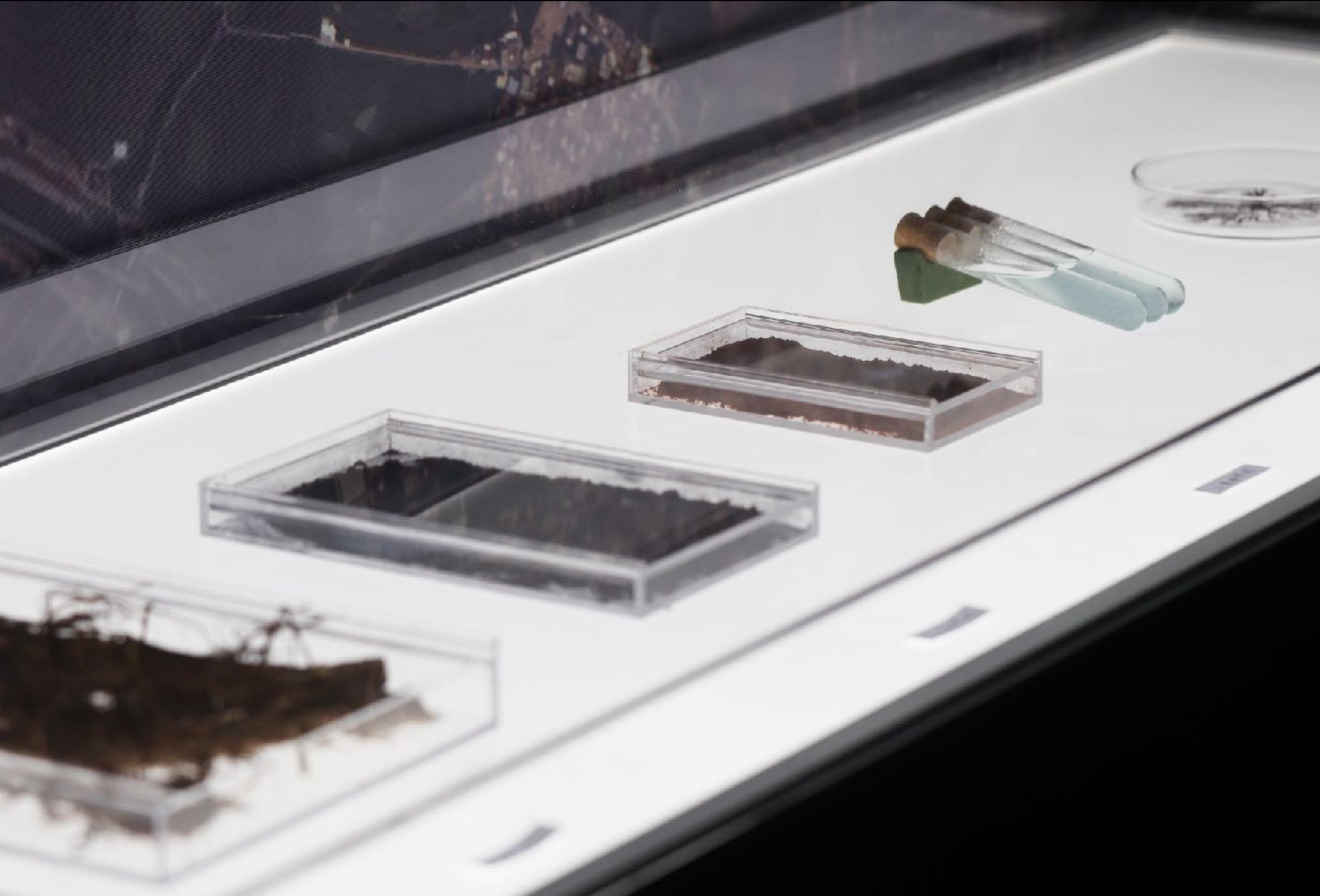
Plant Metallurgy Process: (From Left To Right )- Reed Root, Incomplete Burning of Plant Ash; Fully Burning Plant Ash; Acid Leaching Solution; Electrolytic Copper; Copper Powder
