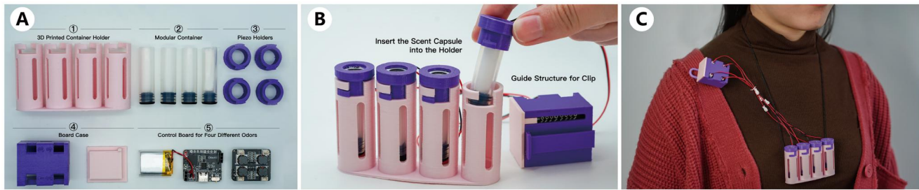
Figure 3. The neck-worn scent-releasing device devised by using OlfackIt.
