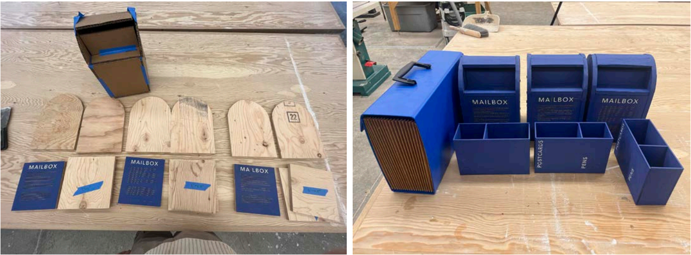
I fabricated each mailbox with plywood. I used a laser cutter to engrave text, and assembled the mailboxes together using a combination of wood glue and mechanical assembly.
