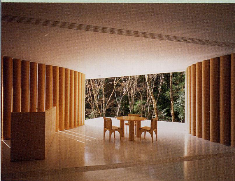
Paper House , interior (with kitchen area at left), permanent building constructed of paper tubes, wood joints, and wood flooring, 1995. Lake Yamanaka, Yamanashi, Japan. All photographs by Hiroyuki Hirai.
