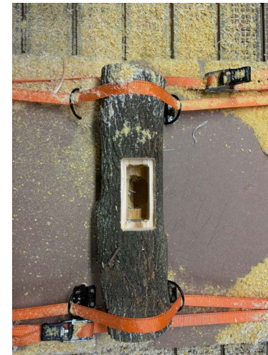
CNC operation for speaker cavity
