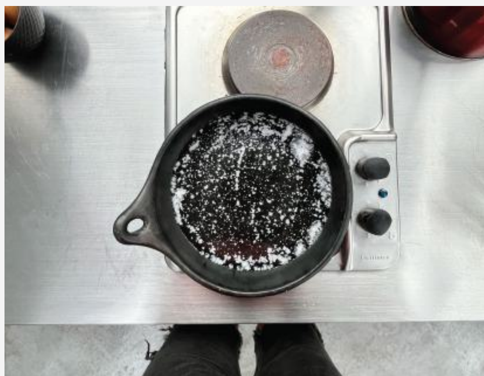
C. While boiling the brine, a dense mass of crystals is formed.
