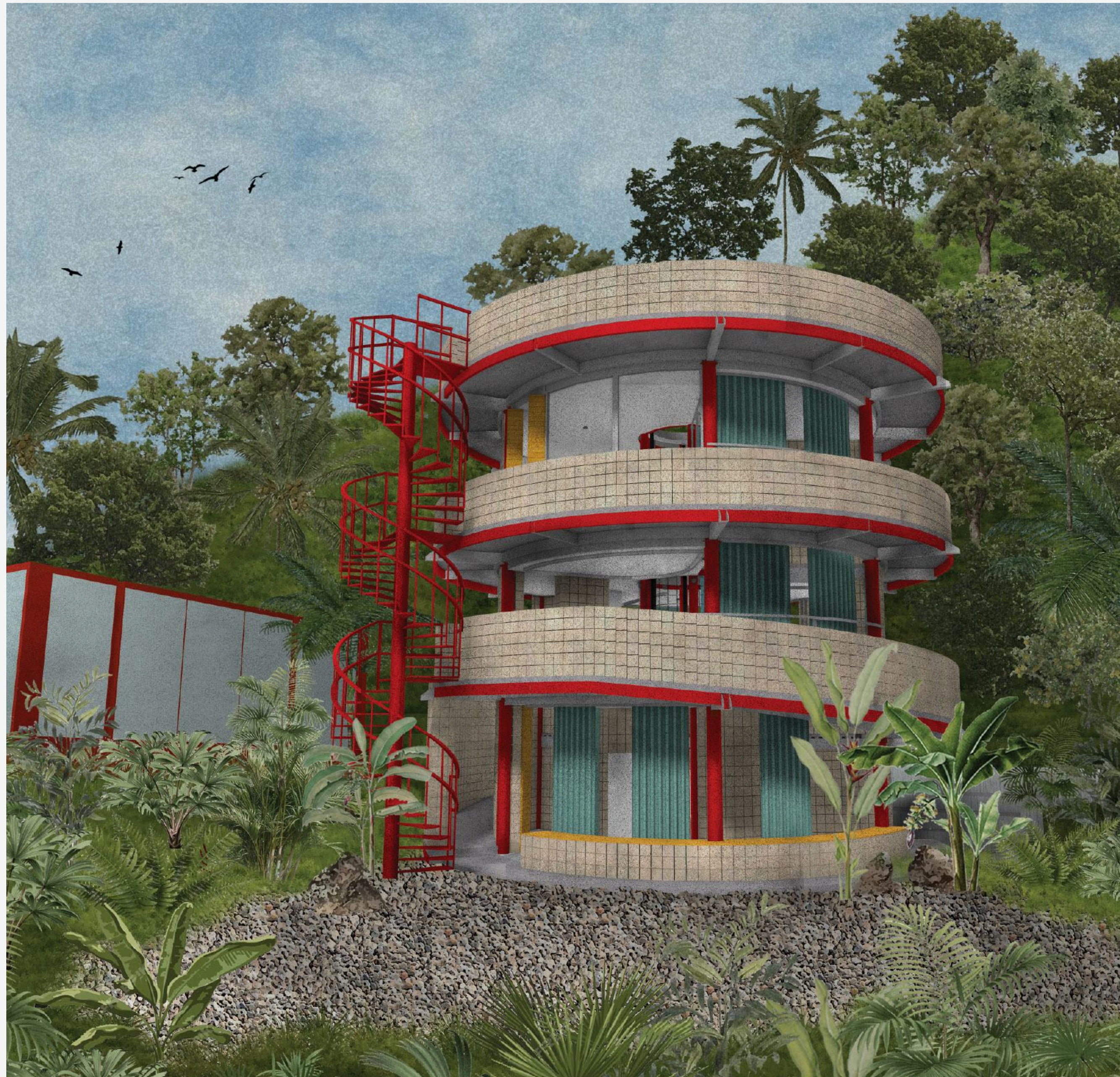
C. TThis house features a circular layout centered around a fireplace. A ramp serves as the main vertical circulation, spiraling through the levels and guiding visitors to take in the surrounding views.
