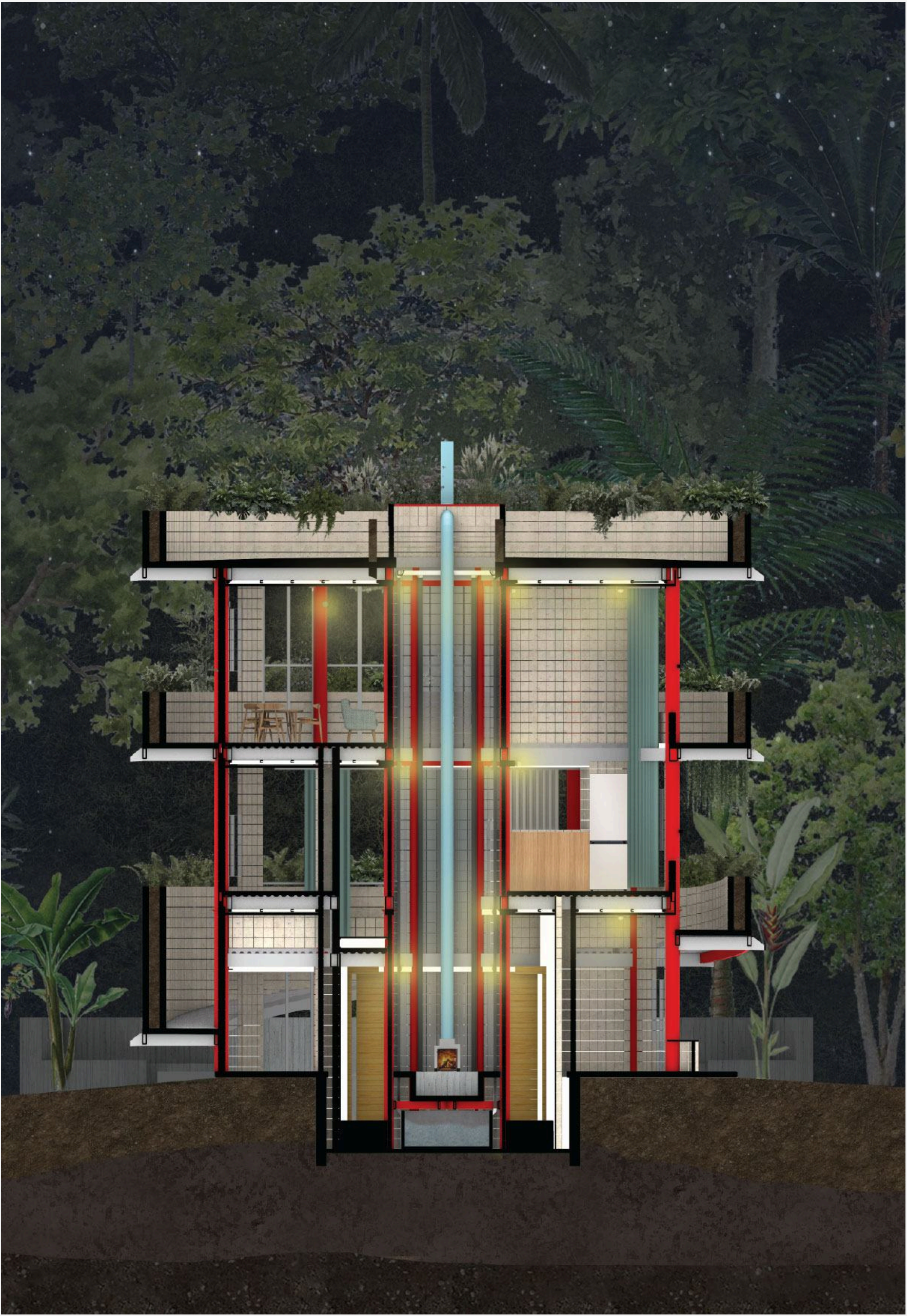
D. This section shows the central space that works as a natural and artificial lamp for the house. It is where the rainwater is collected, stored, and cleaned. It is also a space for contemplating the stars and the moon.moon.
