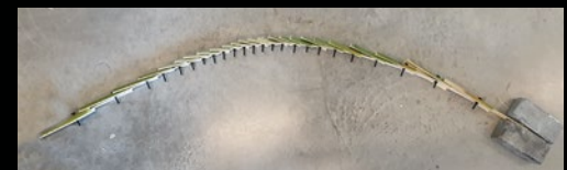
Shingling the tiles on a single flexible bamboo stripe
