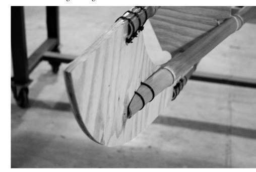
By dry-fitting the bamboo stringers in place, you should be able to approximate the taper needed for a nice fit against the stem and stern. Make sure the bamboo terminates on the stem and stern at the small circles in the drawing mentioned earlier. Draw a line parallel to the stem or stern on the bamboo, remove the stringer, and cut using the jig saw.
