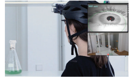
7 Eye-tracking device (prototype 1) detects the gaze direction and position of the visitor
