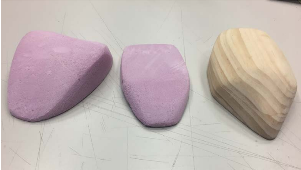
Foam models for lamp shade (to be vacuum formed), and models for individual lids.
