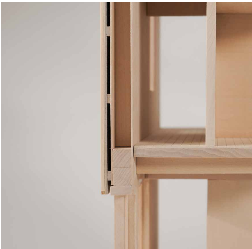
1:20 Carriage Section Model - concrete, wood, paper
