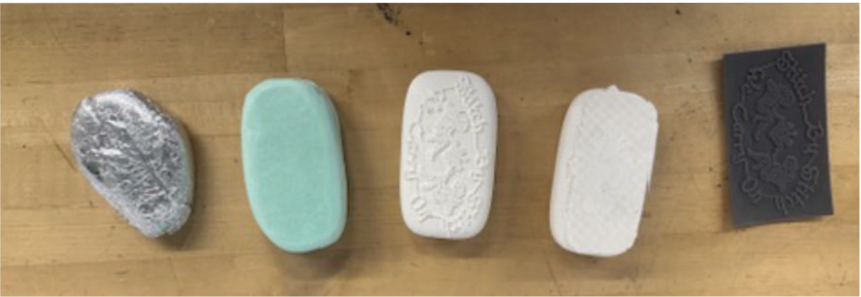
Final prototypes: Foam and Aluminum foil, Foam, 3d printed filament, and Resin
