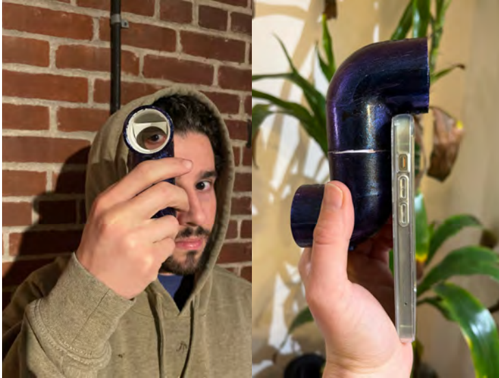
First prototypes made from PVC pipe and craft mirrors
