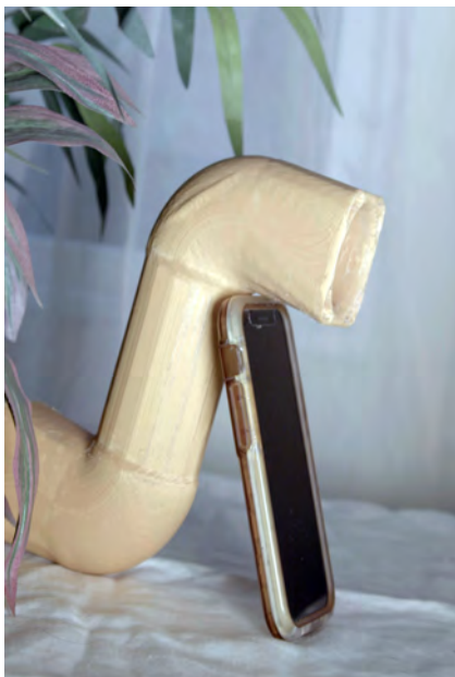
First PLA printed periscope
