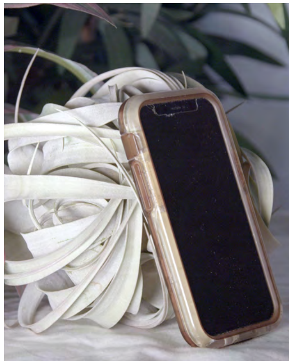
Mirage prototype attached with 3D printed phone case attachment and fishing wire
