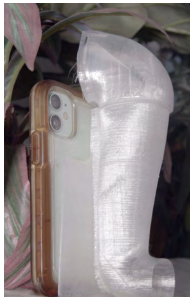
Smaller PLA printed periscope
