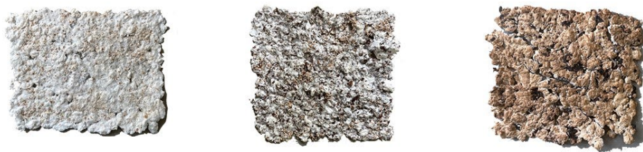
Figure 7: Various produced fabrics: Left: powdered eggshell mixed with paper fabric, Middle: coconut shell mixed with eggshell and paper fabric, Right: ripened banana peel mixed with paper fabric
