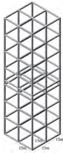
Fig. 5. Isometric projection of a 3D model of the structural frame of Centro Direzionale di Firenze . Image: author
