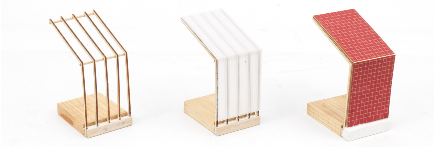
SECTION DETAIL (LEFT) AND WALL TYPOLOGY MODELS (ABOVE), The buildings vary in facade resulting in a patterning of terracotta, glass and open air. The terracotta wall is designed to maximize the collection of water allowing for plants to grow on the wall's surface and irrigating the rest of the site by directing water into the French drain system.
